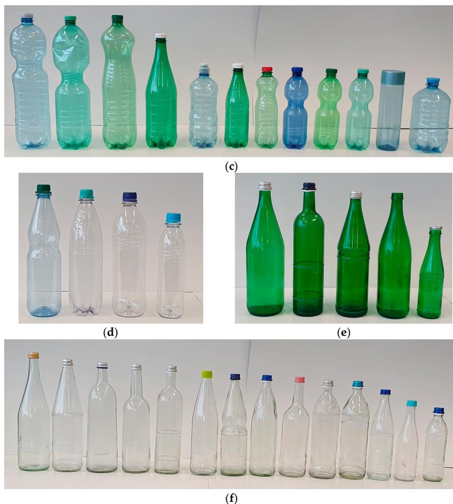
**Figure 3.** Examples of analyzed bottles: (a–c) disposable PET bottles; (d) reusable PET bottles; (e,f) reusable glass bottles.
