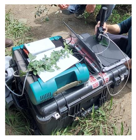
**Figure 2.** Reflectance data collection over a leaf, during fieldwork, with a spectroradiometer ASD FieldSpec<sup>®</sup> 4.
