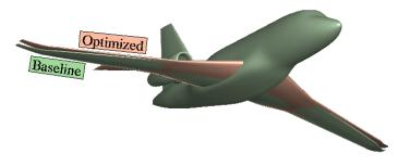
**Figure 20.** Aerostructural optimization with varying structural model (OptR9), using PUMA: Comparison of the wing shape of the baseline GBJ and the outcome of OptR9.
