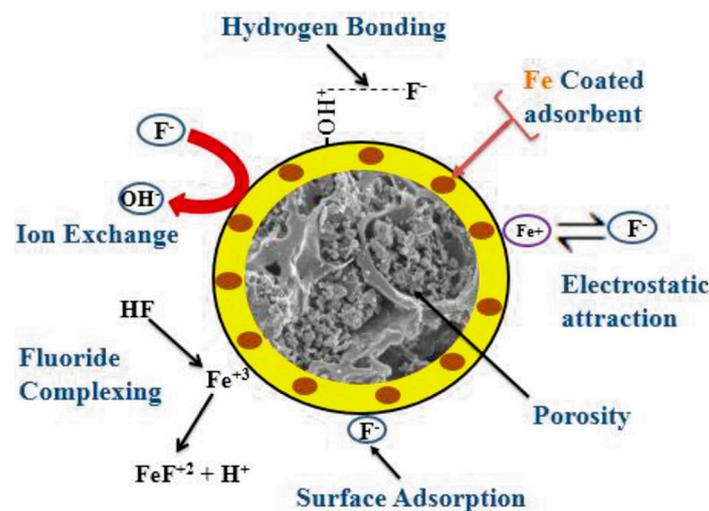
**Figure 7.** Possible adsorption mechanism of fluoride on MPPAC-500 [60] (no special permission is required to reuse).
