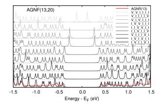
**Figure 5.** Density of states of AGNF(13,20) with two  $CH_2$  groups on each cap. All of the different positions of double H saturations are considered. The larger the vertical shift of the DOS, the less stable the corresponding conformation and the lighter the shade of gray. Note that in the most stable configuration, the HOMO–LUMO separation of the flake became slightly larger than the gap of AGNR(13), whose DOS is depicted in red.
