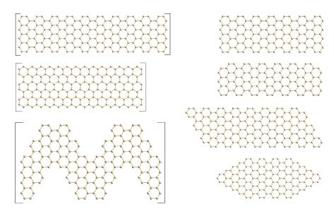
**Figure 1.** Stick-and-ball representation of graphene nanoribbons and graphene nanoflakes. **Left** panels, from top to bottom: *armchair, zigzag,* and *chevron* nanoribbons. **Right** panels, from top to bottom: *hammer* (9,7), *hammer* (8,7), *cutter,* and *pencil* nanoflakes cut from *armchair* nanoribbons.
