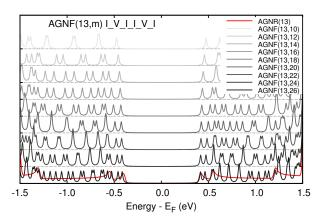
**Figure 4.** Density of states of the AGNF(13,*m*) series (m = 10 - 26) (in shades of gray), plus the DOS of the infinite AGNR(13) ribbon (depicted in red). The data are shifted according to the length of the flake; the smaller *m* is, the larger the vertical shift is and the lighter the curve is. In all systems, we adopted the most stable saturation stoichiometry with two CH<sub>2</sub> groups at each cap and the most stable conformation of hydrogens, i.e.,  $I_VI_IV_I$ .
