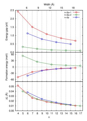
**Figure 2.** Properties of graphene nanoribbons with different widths *n*. Data are reported in red, green, and blue for the n = 3p + 1, n = 3p + 2, and n = 3p families, respectively. **Top** panel: energy gaps; **middle** panel: formation energies (also called edge energies); **bottom** panel: variation in the optimized unit cell length of AGNRs with respect to an orthorhombic supercell of graphene with L = 4.29 Å and hosting four C atoms per unit cell.
