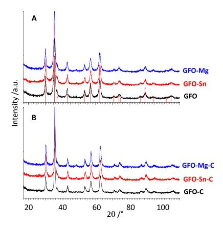
**Figure 1.** X-ray diffraction patterns of pure and doped GFO samples obtained before (**A**) and after (**B**) carbon coating. In (**A**), the expected reflections of GeFe<sub>2</sub>O<sub>4</sub> spinel (card N. 25-0359) are reported as red bars.
