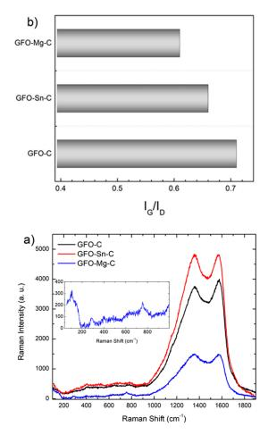
**Figure 3.** Room temperature Raman spectra of the carbon-coated samples. (a) Inset: zooming of the low energy activity for the GFO-Mg-C sample. (b) IG/ID values calculated for each investigated sample.
