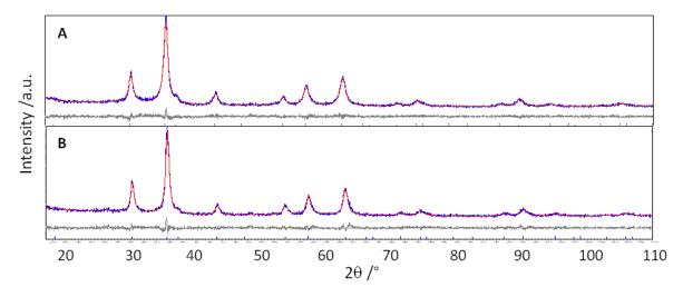
**Figure 2.** Rietveld refinement of GFO-Sn (**A**) and GFO-Sn-C (**B**) patterns. The experimental patterns (blue) and the calculated ones (red) are compared; at the bottom, the difference curve (grey) and the bars of the calculated peak positions are reported.
