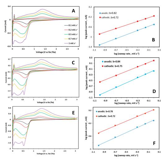
**Figure 6.** CV curves at various sweep rates and b values calculated by considering the relation between Ip and  $\nu$  for GFO-C (**A**,**B**), GFO-Sn-C (**C**,**D**), and GFO-Mg-C (**E**,**F**) samples.
