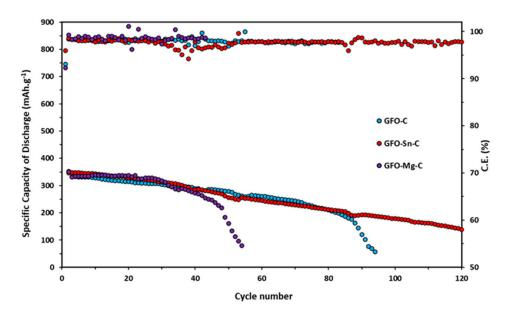
**Figure 8.** Discharge capacity values during long-term cycling at 0.2 C for all samples. The Coulombic efficiencies (C.E.) are also shown.
