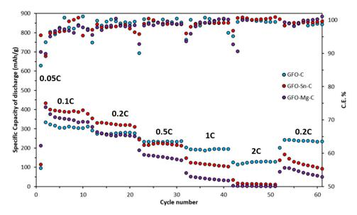
**Figure 7.** Discharge capacity values of the carbon-coated samples at different C rates. In addition, the Coulombic efficiency (C.E.) is also shown.
