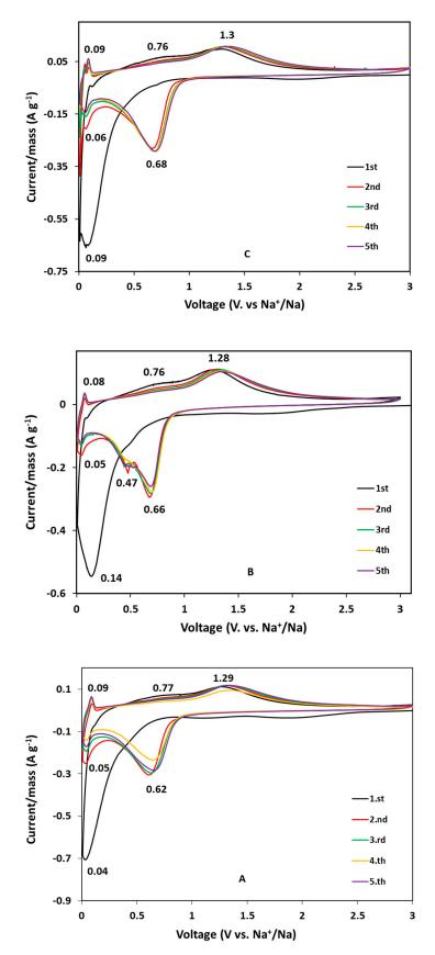
**Figure 5.** Cyclic voltammograms of the carbon-coated GFO samples: (**A**) GFO-C; (**B**) GFO-Sn-C; and (**C**) GFO-Mg-C.
