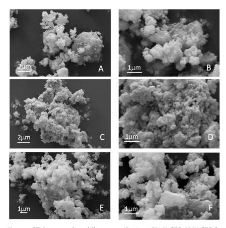
**Figure 4.** SEM micrographs at different magnifications of (**A**,**B**) GFO, (**C**,**D**) GFO-Sn, and (**E**,**F**) GFO-Mg samples.
