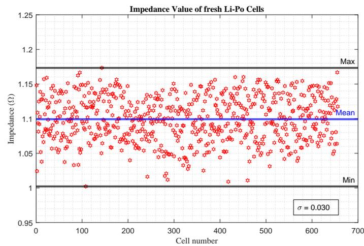
**Figure 4.** DC internal resistance measurement results for 700 fresh Li-Po Cells in the same SOC to show the variation after formation cycling with a variation coefficient (standard deviation/mean) of 0.030. The minimal and maximal resistances that define the window are 1 m $\Omega$  and 1.17 m $\Omega$ , respectively.
