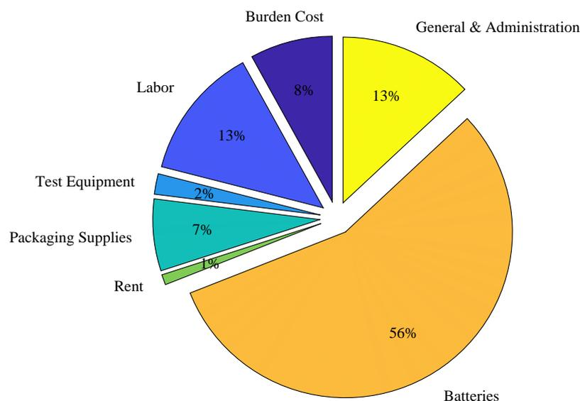
**Figure 14.** Cost breakdown of second-life stationary battery packs, highlighting the significant impact of various factors on total battery pack costs, with battery procurement representing the largest portion. Labor costs, including employment and overhead, also contribute significantly, as do materials required for repackaging used EV modules into battery packs (adapted with permission from [156,157]).
