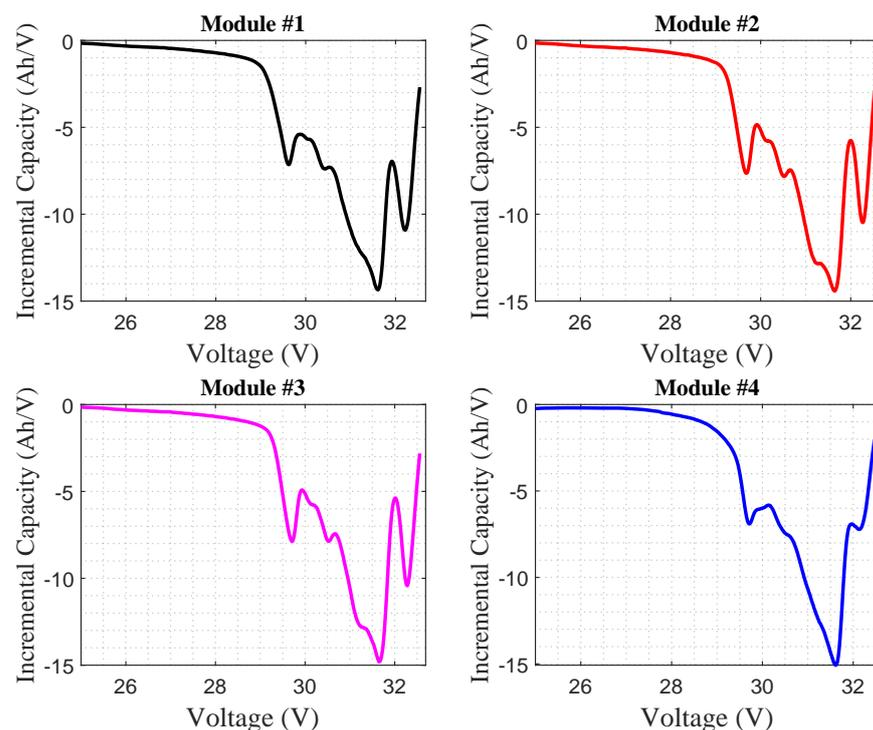
**Figure 6.** Measured ICA curve of four battery modules from an HEV during the discharge process. Module 4 shows a flattening of the right-most trough, indicating the discrepancy of its SOH relative to the other 3 modules.
