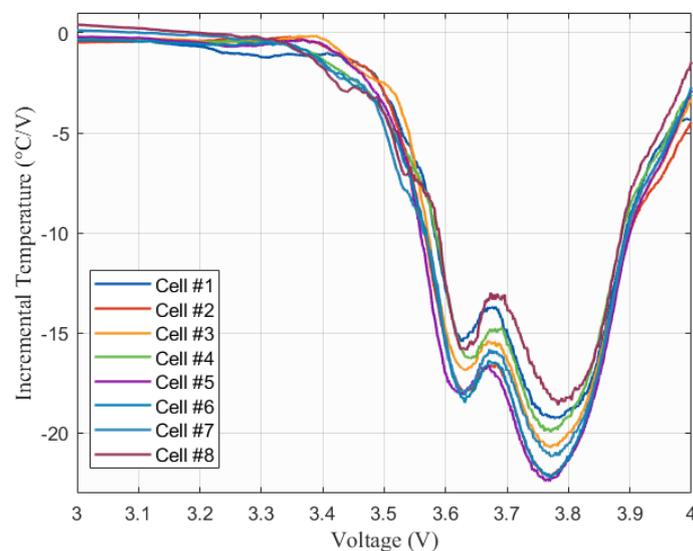
**Figure 9.** Differential thermal voltammetry analysis of a module with 8 LMO cells. Three features can be derived from the valley values, peaks, and the position of each peak, which can be analyzed separately to be linked to the degradation of the battery. It is evident that cells 5 and 6 in the pack show the lowest differential temperature while cells 7 and 8 have the highest.
