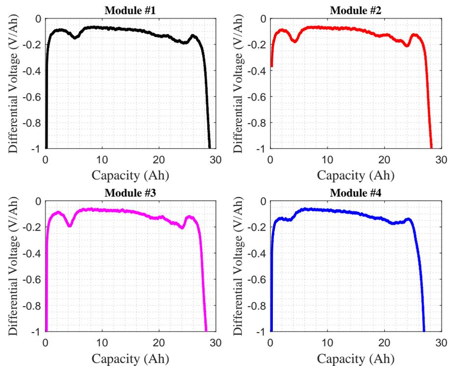
**Figure 7.** Measured DVA curve of four modules from the same HEV battery pack as in Figure 6 during the discharge process. The fading of the right-most peak in Module 4 and its impact on SOH is evident in the figure.
