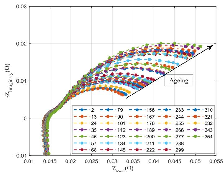
**Figure 11.** Nyquist plots for a single NMC cell under a specific cycling pattern of 4C discharge current rate and 80% DOD at room temperature for a measurement frequency between 20 Hz and 100 kHz. The results show a shift to the right and top of the mid-frequency spectrum caused by the degradation inside the battery with increasing cycle index, indicating this frequency range has a good correlation with the battery SOH.
