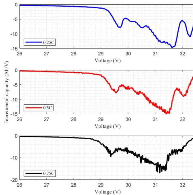
**Figure 8.** ICA curves at different  $C_{rate}$  for module 1 from the same HEV battery pack as Figures 6 and 7.
