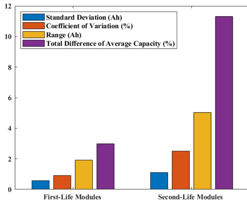
**Figure 13.** Comparison of capacity data between first- (left) and second-life (right) modules based on capacity measurement data of 32 second-life modules and ten new modules (data adapted from [19]).
