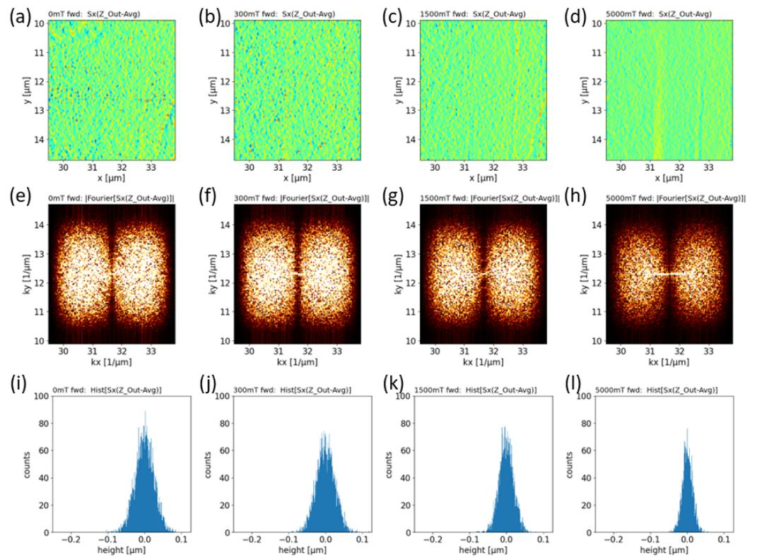
**Figure A2.** Statistical methods described in the main text applied to the Sobel gradient for the forward scanning direction. Noise plot generated by subtracting the total spatial average for (a) 0 T, (b) 0.3 T, (c) 1.5 T and (d) 5 T. Fourier transform of corresponding (e) 0 T, (f) 0.3 T, (g) 1.5 T and (h) 5 T noise plots. Histograms of corresponding (i) 0 T (j) 0.3 T, (k) 1.5 T and (l) 5 T noise plots.
