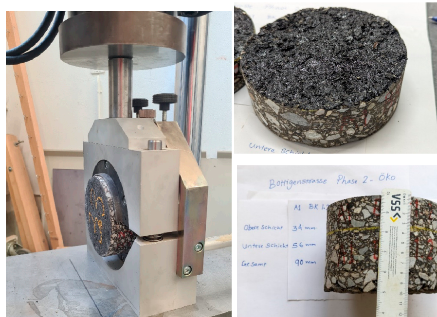
Figure 10. Shear bond test set up (left) and the core before and after the test (right).
