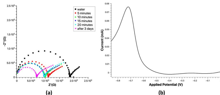
**Figure 1.** Direct sensing of n-ZnO effect in aqueous fluids. (a) Time-dependent analysis of the impedance of solution containing n-ZnO. (b) Preliminary voltammetric determination of zinc ions.
