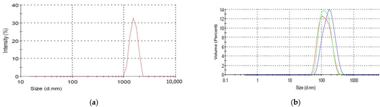
**Figure 5.** Particle size distribution of (a) microcapsules with a polyurea shell and DCOIT biocide load in the core [96] and (b) microcapsules with a shell made of silicon dioxide nanoparticles and a core of polymethacrylate containing DCOIT: red line—before filtration; green line—after polymerization, blue line—after polymerization [81].
