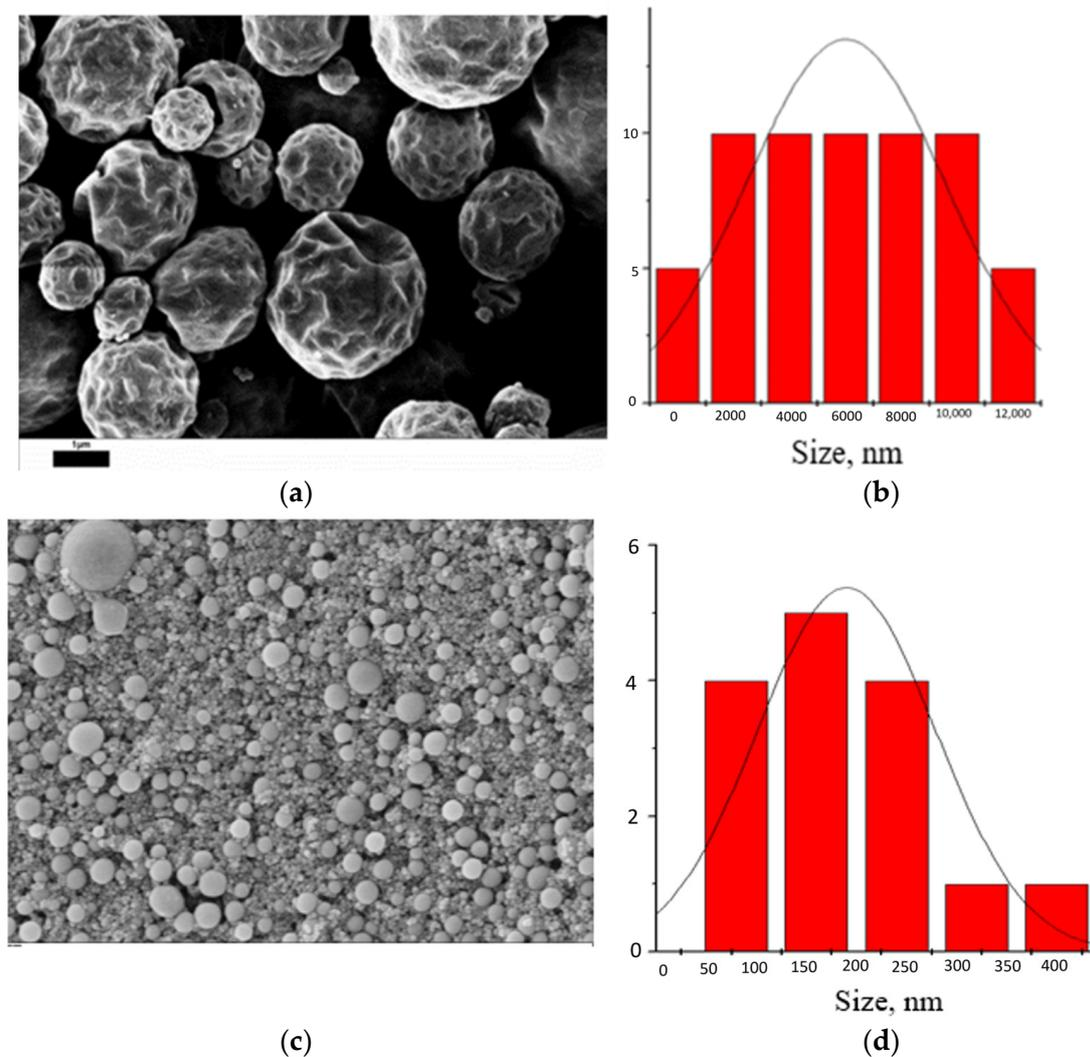
**Figure 6.** SEM micrographs and particle size distribution curves: (a,b) microcapsules with a shell made of silicon dioxide nanoparticles and a core of polymethacrylate containing DCOIT [40]; (c,d) microcapsules with a polyurea shell with DCOIT biocide in the core [96].
