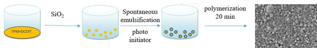
**Figure 2.** Schematic representation of the production of microcapsules by using nanoparticles [81].
