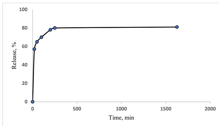
**Figure 7.** Biocide release rate from micro- and nanocapsules with a shell made of silicon dioxide nanoparticles and a core of polymethacrylate with DCOIT [81].
