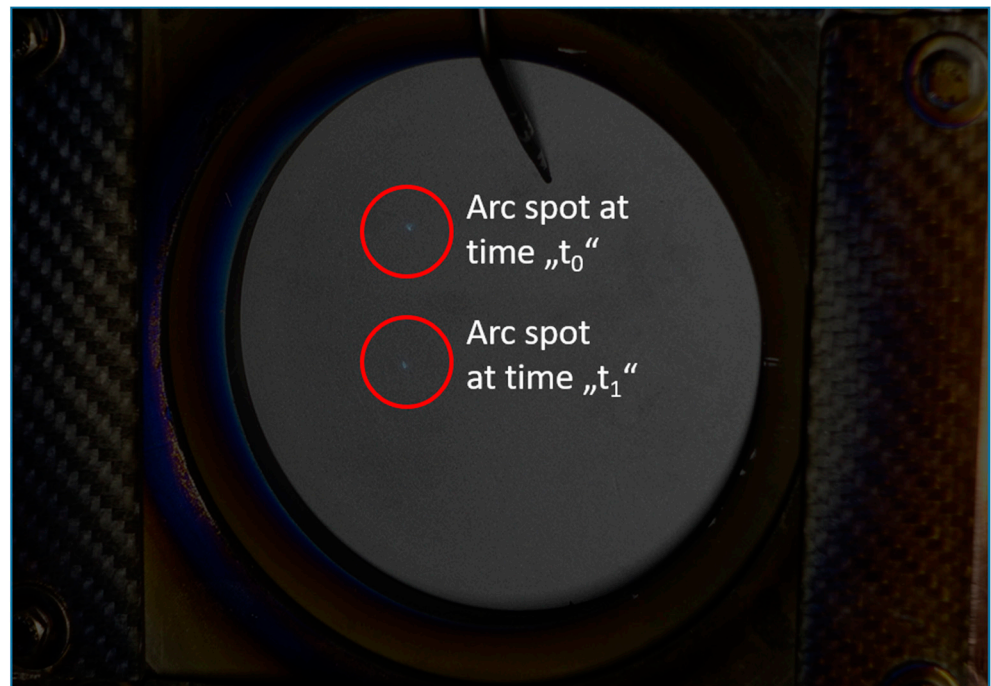
Figure 6. Short time photographs of arc spot positions to determine the distance between subsequent positions of a random walk motion. Processing conditions: Circular cathode, Current = 20 A.
