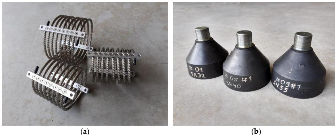
**Figure 1.** Investigated wire rope shockmounts (a) and elastomer shockmounts (b), one of each type.
