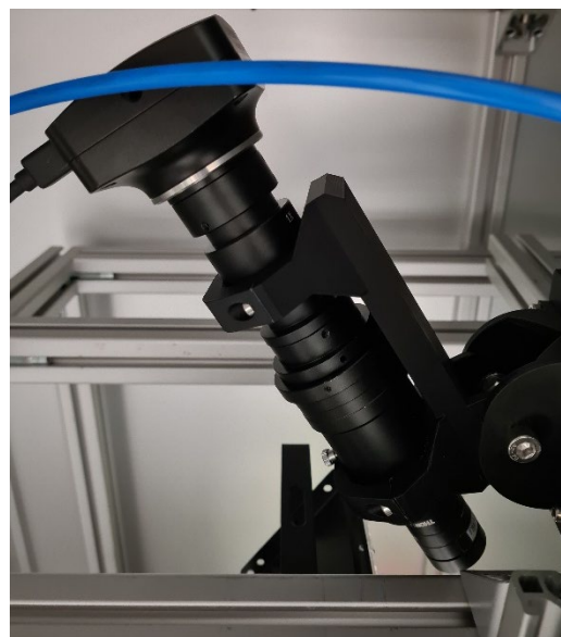
Figure 7. Camera system for optical analysis of the process action point.
