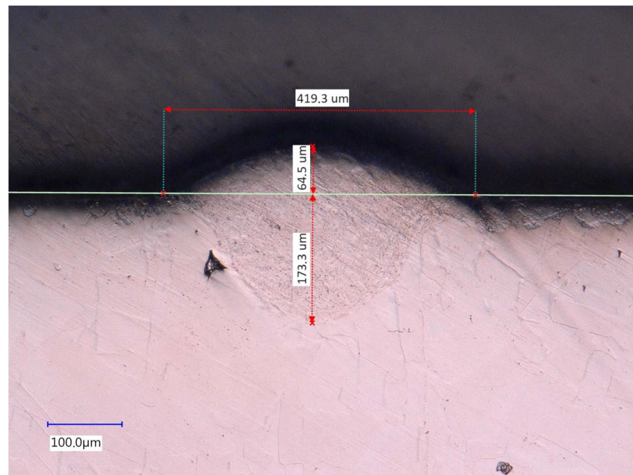
Figure 11. Micrograph of 20 welded tracks placed on top of each other.
