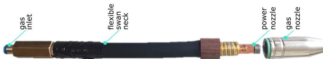
Figure 5. Structure of the shield gas supply.
