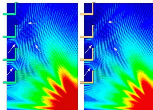
Figure 7. Acoustic pressures around the balcony for both uniform (Case 2, (left)) and jagged (Case 4, (right)) ledge designs.
