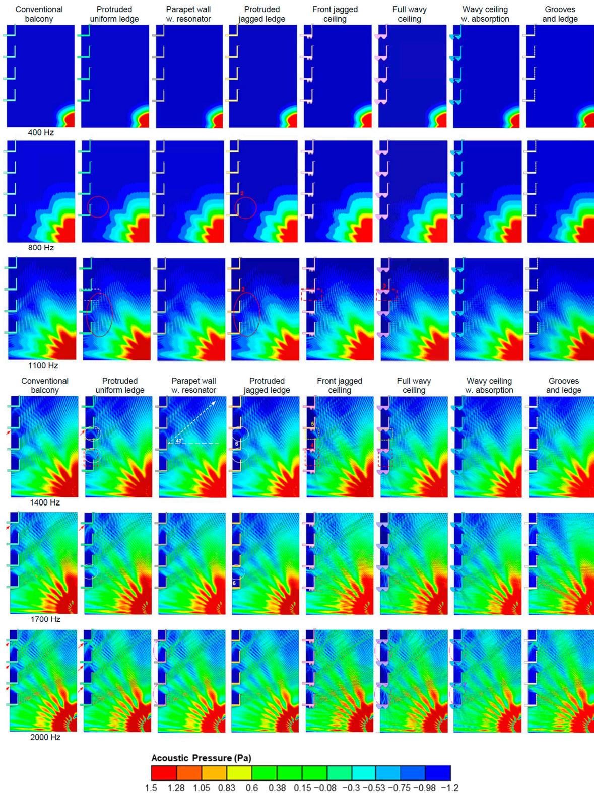
**Figure 3.** Acoustic pressure (Pa) contour plots at different frequencies for the various balcony designs.
