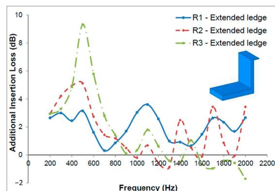
**Figure 4.** Additional IL characteristics for balcony with protruded parapet ledge (Case 2).
