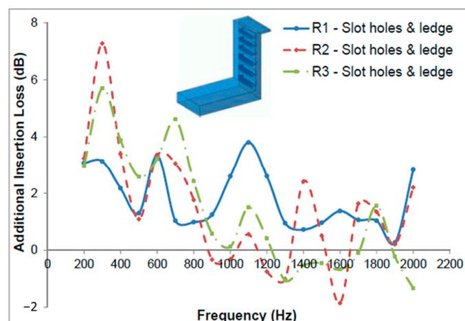
**Figure 14.** Additional IL characteristics for the balcony wall with ledge and grooves (Case 8).
