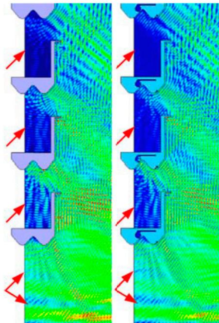
**Figure 13.** Acoustic pressure contours around the balcony, for both wavy ceiling designs untreated (Case 6, **left**) and treated (Case 7, **right**) with additional absorption.
