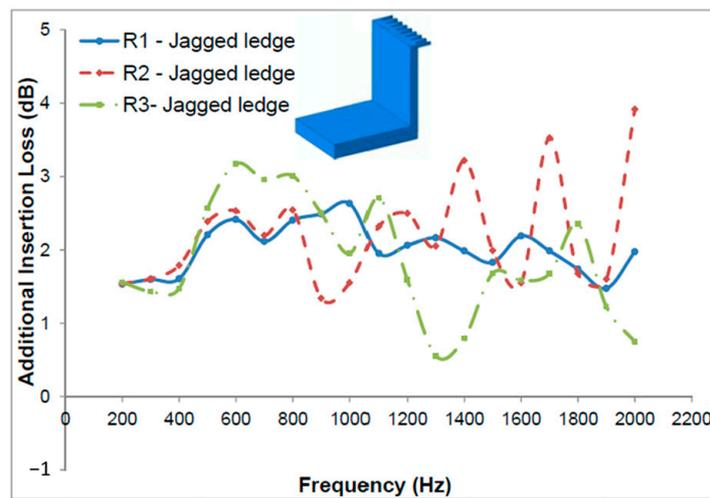
Figure 6. Additional IL characteristics for balcony with jagged ledge (Case 4).
