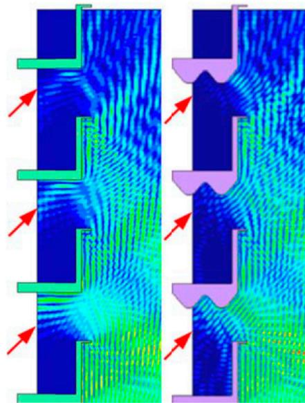
**Figure 11.** Acoustic pressure contours around the balcony for both uniform ledge (Case 2, (left)) and full wavy ceiling (Case 6, (right)) designs.
