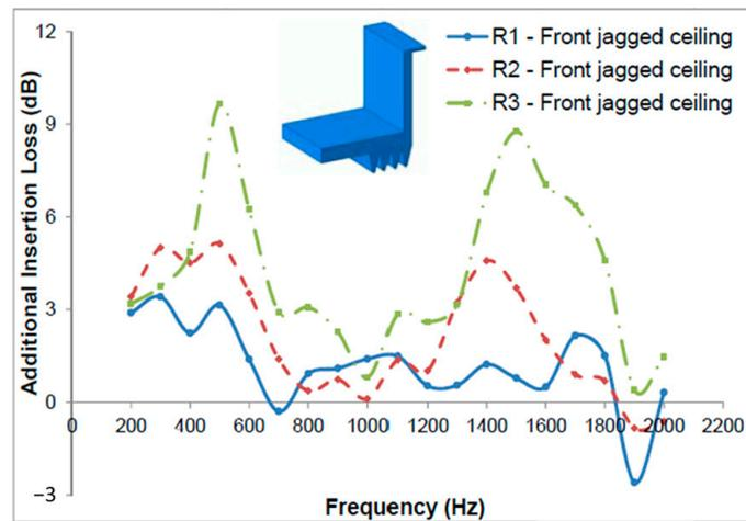
Figure 8. Additional IL characteristics for balcony with front jagged ceiling (Case 5).
