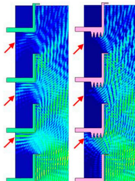
Figure 9. Acoustic pressure contours around the balcony for both uniform ledge (Case 2, (left)) and front jagged ceiling (Case 5, (right)) designs.
