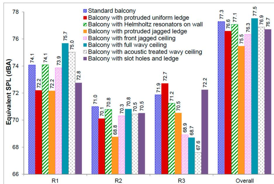
**Figure 18.** Equivalent sound pressure level in different regions for the various balcony designs.
