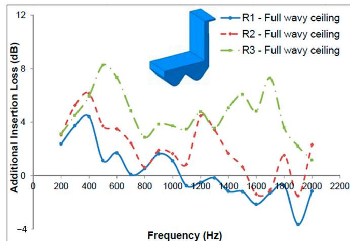
Figure 10. Additional IL characteristics for the balcony with full wavy ceiling design (Case 6).
