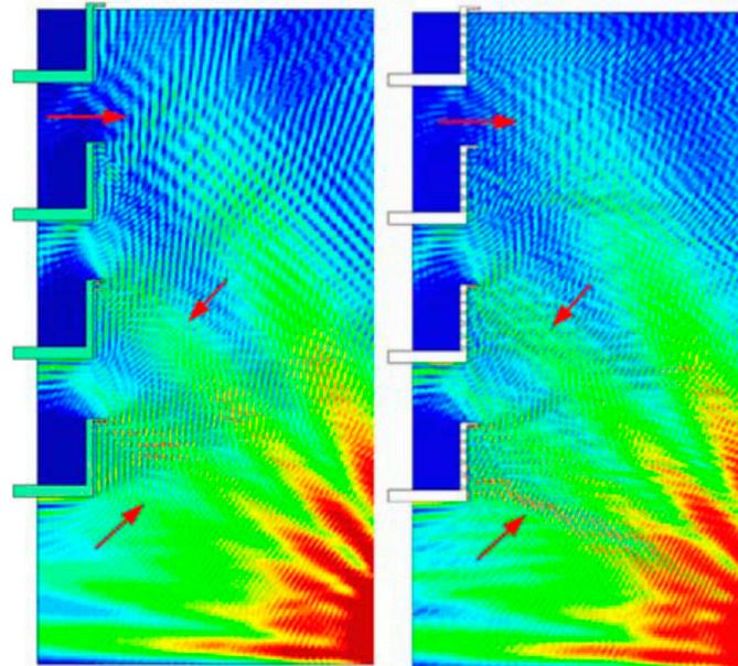
**Figure 15.** Acoustic pressure contours around the balcony for both uniform ledge (Case 2, (left)) and grooved wall (Case 8, (right)) designs.
