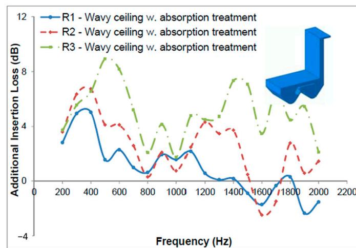
**Figure 12.** Additional IL characteristics of the balcony with a wavy ceiling treated with additional absorption (Case 7).
