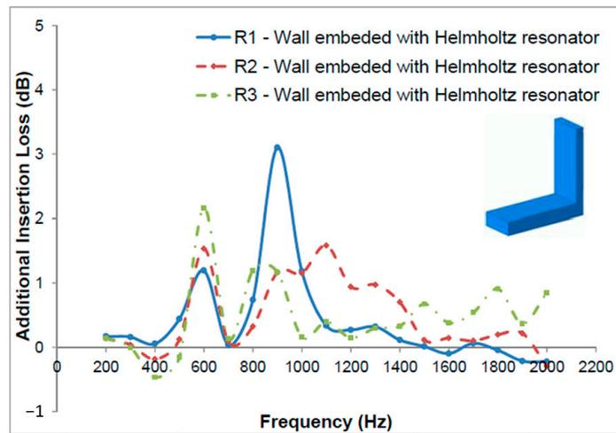
Figure 5. Additional IL characteristics for balcony with parapet embedded with Helmholtz resonator (Case 3).
