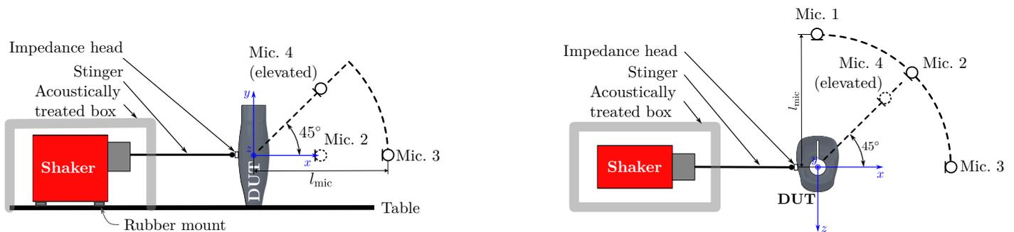
**Figure 8.** Sketch of the experimental setup for the microphone measurements. Mic. 1, 2, and 3 are located in the  $x/z$  plane. Mic. 4 is at  $45^\circ$  elevation above mic. 2. The coordinate system's origin is located in the center of the device under test (DUT), such that the excitation force vector lies inside the  $x/z$  plane.
