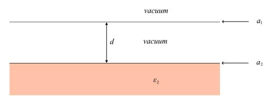
**Figure 2.** The Chern–Simons layer defined by  $a_1$  is separated by a distance *d* from a dielectric half-space, with the boundary Chern–Simons layer defined by  $a_2$ . The permittivity of a dielectric half-space is  $\varepsilon_2$ .
