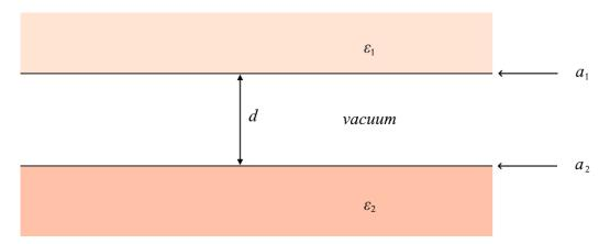
**Figure 1.** Two dielectric half-spaces with Chern–Simons boundary layers are separated by a distance *d*. The permittivity of the upper dielectric half-space is  $\varepsilon_1$ ; the permittivity of the lower dielectric half-space is  $\varepsilon_2$ . The upper Chern–Simons boundary layer is defined by  $a_1$ ; the lower Chern–Simons boundary layer is defined by  $a_2$ .
