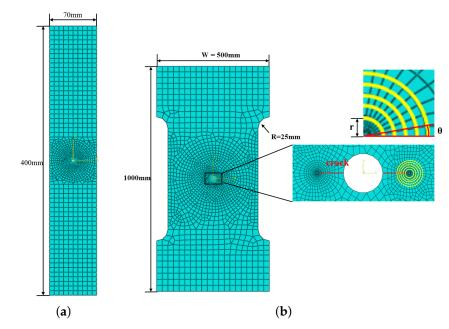
**Figure 3.** (a) Small wall panel, (b) big wall panel. The yellow lines highlight the mesh layers drawn at the crack tip, *r* is the radius size of the first layer of the mesh, and  $\theta$  is the angle size of the mesh divided around the front of the crack.
