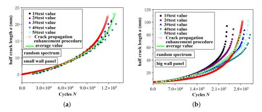
**Figure 6.** (a) Load spectrum a - N curve of small wall panel. (b) Load spectrum a - N curve of big wall panel.
