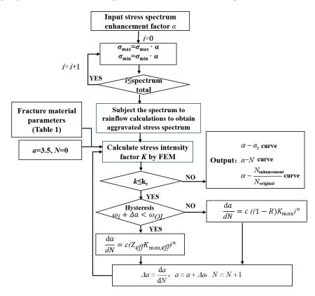
Figure 2. Flow chart of random load spectrum crack growth enforcement calculation program.
