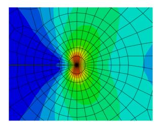
Figure 4. Crack tip finite element stress.
