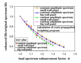
**Figure 10.** Load spectrum enhancement  $\alpha - N_{enhancement} / N_{original}$  original spectrum curves.
