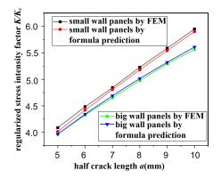
**Figure 7.** a - K curve with different calculation methods.
