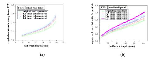
**Figure 8.**  $a - K/K_c$  curves with differnt enhancement factors of (**a**) small wall panel and (**b**) big wall panel.
