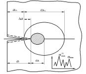
**Figure 1.** The diagram of Willenborg–Chang crack model with a random load spectrum. The crack with full lines is the old crack with a length of  $a_{OL}$ , and the dash line crack is a new one with a length of  $a_{OL} + \Delta a$ .
