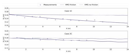
Figure 2. Simulated wave heights over a rippled bed, considering energy loss resulting from friction at the bottom (solid lines) and experimental measurements (points) of [66]. The dashed line denotes simulation results without considering the effect of bottom friction.
