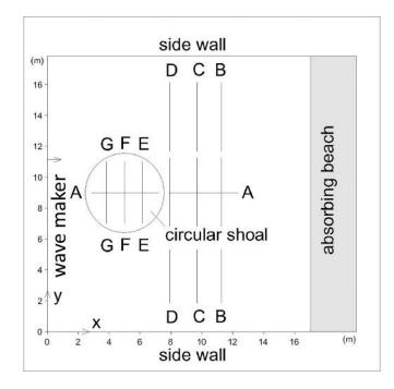
Figure 4. Layout of the [68] experiments.
