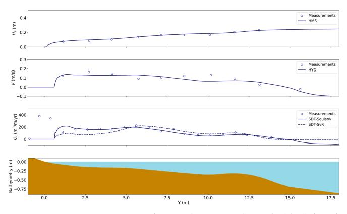
**Figure 13.** Comparison of experimental measurements and numerical model results for significant wave heights, longshore current speeds, and sediment transport rates of test BC1. The bathymetry of the coastal profile is given at the bottom of the Figure.
