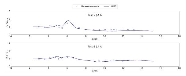
**Figure 5.** Normalized wave heights as calculated by the HMS model (solid line) and as measured (points) for Test 5 of the [68] experiments, at the longitudinal transect A-A.
