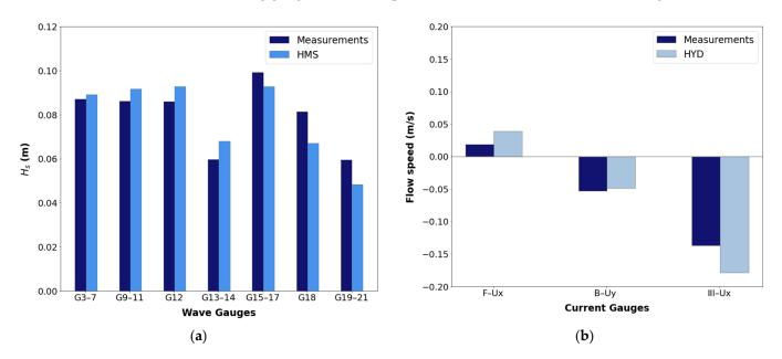
The comparison between the computed wave heights and current speeds at selected measuring gauges with the experimental measurements is shown in Figure 10.
