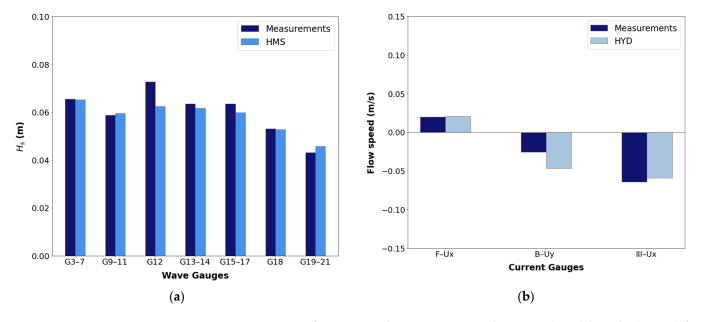
**Figure 11.** Comparison of experimental measurements and numerical model results (Test 35) for (a) wave heights and (b) current speeds.
