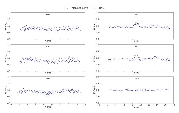
**Figure 7.** Normalized wave heights as calculated by the HMS model (solid line) and as measured (points) for Test 6 of the [68] experiments, at six transverse transects.
