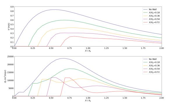
**Figure 17.** Cross-shore distribution of longshore current (**top**) and longshore sediment transport rate (**bottom**) for a 1:10 beach (Case 1b) without a seawall and various placements of a seawall along the surf zone.
