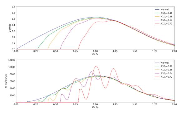
**Figure 19.** Cross-shore distribution of longshore current (**top**) and longshore sediment transport rate (**bottom**) for the case of a 1:50 (Case 2b) beach without a seawall and various placements of a seawall along the surf zone.
