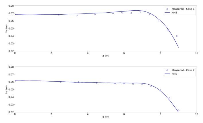
**Figure 3.** Computed values (solid line) by HMS and experimental data (circular markers) by [67], for Case 1 (**top**) and Case 2 (**bottom**).
