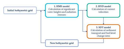
Figure 1. Flowchart of the implementation sequence of numerical models.
