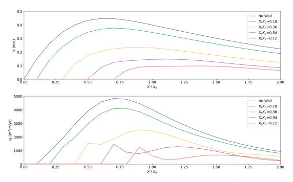
**Figure 16.** Cross-shore distribution of longshore current (**top**) and longshore sediment transport rate (**bottom**) for a 1:10 beach (Case 1a) without a seawall and various placements of a seawall along the surf zone.
