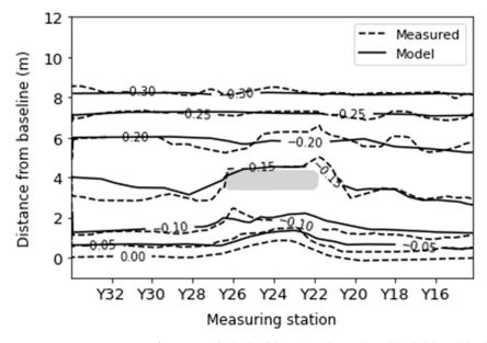
**Figure 15.** Comparison of measured (dashed lines) and simulated (solid lines) bed elevations at the end of the test T1C1 of the experiments conducted in [74].
