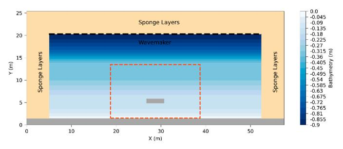
**Figure 14.** Numerical layout of the T1C1 experiment of [74]. The orange dashed polygon denoted the area where the morphological bed evolution results will be evaluated.
