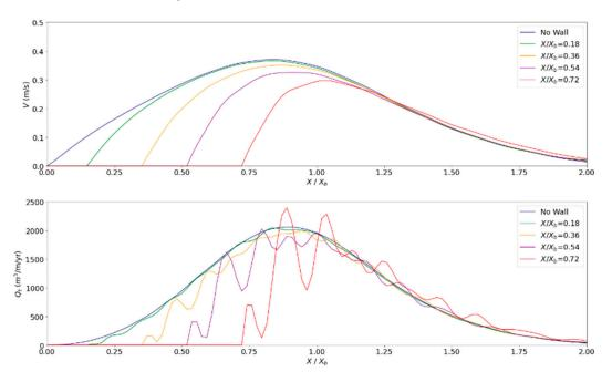
**Figure 18.** Cross-shore distribution of longshore current (**top**) and longshore sediment transport rate (**bottom**) for the case of a 1:50 (Case 2a) beach without a seawall and various placements of a seawall along the surf zone.
