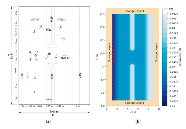
**Figure 8.** Layout of the [72] experiment (**a**) with positions of measuring wave (#1-21) & current speed (F, B and III) gauges and (**b**) bathymetry for the numerical implementation.
