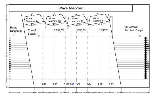
Figure 12. Layout of the LSTF experiment of [74] (adapted from [75]).
