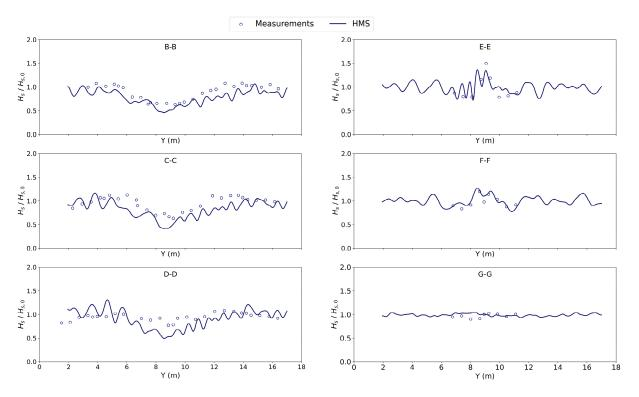
**Figure 6.** Normalized wave heights as calculated by the HMS model (solid line) and as measured (points) for Test 5 of the [68] experiments, at six transverse transects.
