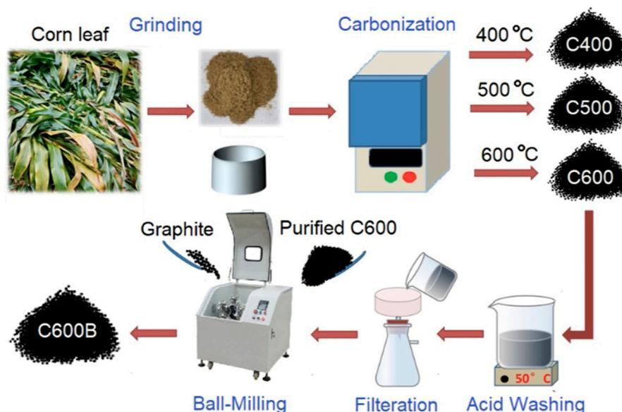
**Figure 11.** Scheme of carbon material preparation from corn leaf. Adapted from reference [18].
