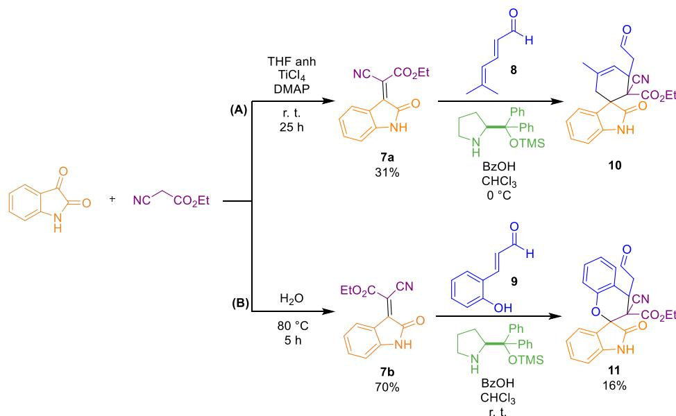
**Scheme 3.** 3-Methylenindolin-2-one synthesis and spirooxindole formation. (A) Knoevenagel condensation between isatin and ethyl cyanoacetate yielded **7a**, and subsequent organocatalytic Diels–Alder reaction to yield spirooxindole **10**. (B) Knoevenagel condensation between isatin and ethyl cyanoacetate yielded **7b**, and organocatalytic oxa-Michael–Michael reaction for the obtention of spirooxindole **11**.
