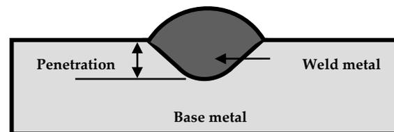
Figure 1. Depth of penetration of weld bead.
