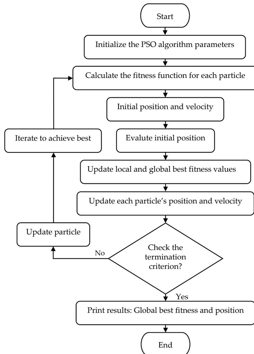
**Figure 3.** Flow chart of PSO algorithm.
