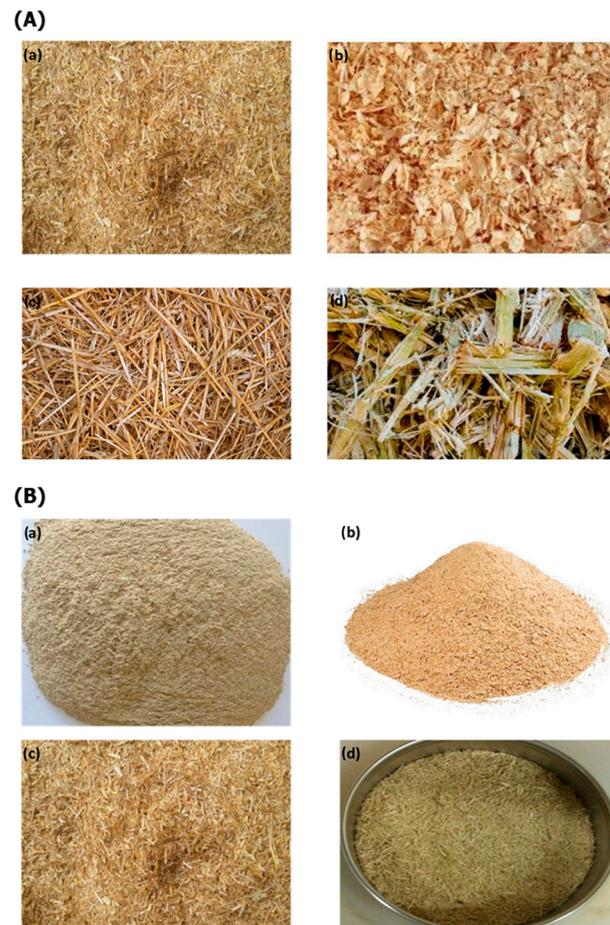
**Figure 2.** Raw materials (A) before grinding and (B) after grinding: (a) rice husk; (b) saw dust; (c) wheat straw; (d) bagasse.
