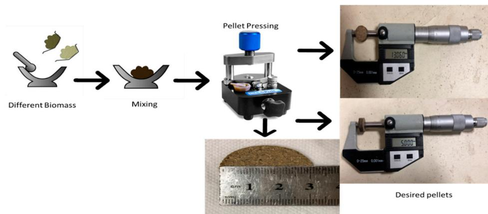
**Figure 3.** Method of preparation of desired pellets.
