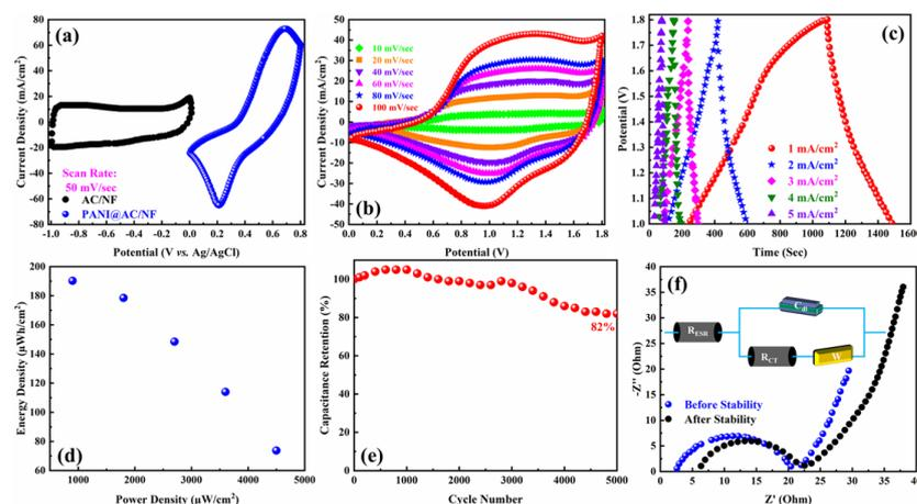
**Figure 3.** (a) CV curves of electrodes, (b) CV curves, (c) GCD profiles, (d) Ragone plot, (e) capacitance retention, and (f) Nyquist plots of the PANI@AC/NF//AC/NF ASC.
