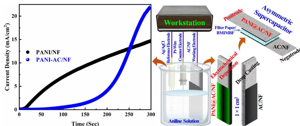
**Figure 1.** Amperometric response on a bare and AC-modified NF substrate and the corresponding PANI@AC/NF//AC/NF ASC.
