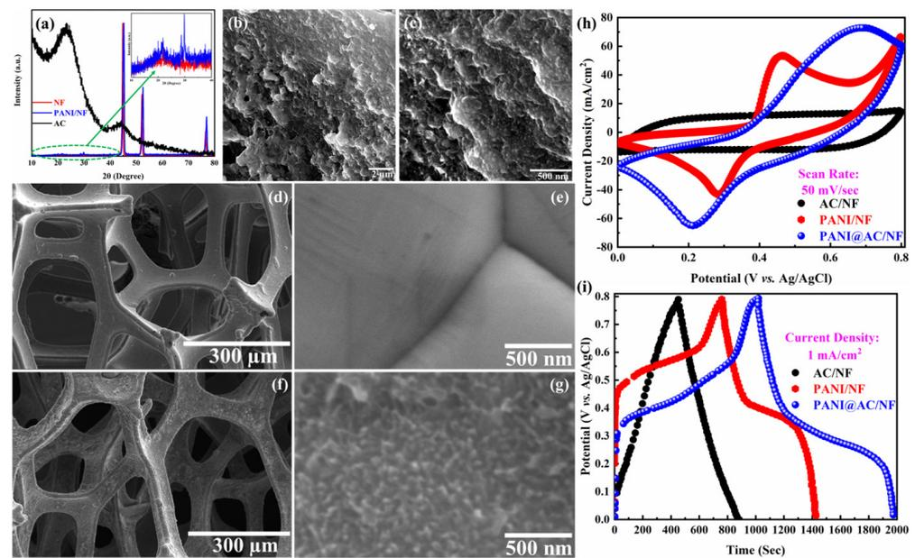
**Figure 2.** (a) XRD patterns and FESEM images of (b,c) AC, (d,e) NF, and (f,g) PANI/NF. (h) CV curves and (i) GCD profiles various prepared electrodes.
