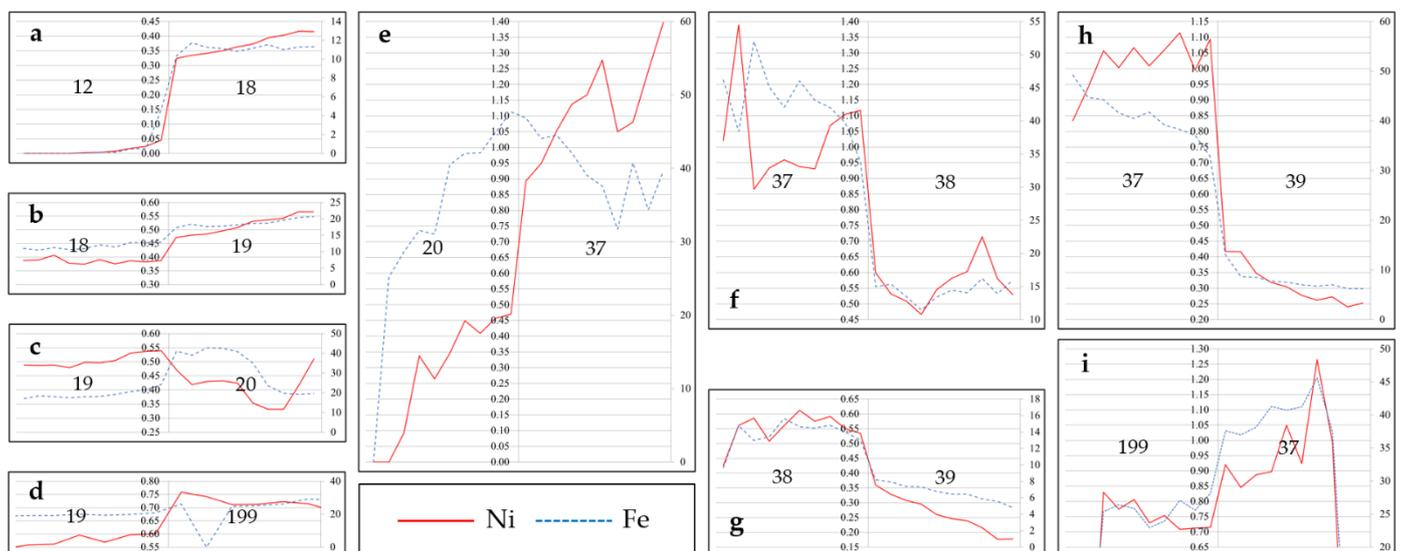
**Figure 4.** Contact profile graphs between various domains of the Tsouka deposit. The middle vertical axis shows mean Ni% grades of distance intervals on either side of the contact, while the right vertical axis shows corresponding mean Fe% grades. The horizontal axis starts and ends 10 m before and after the boundary between the two domains.
