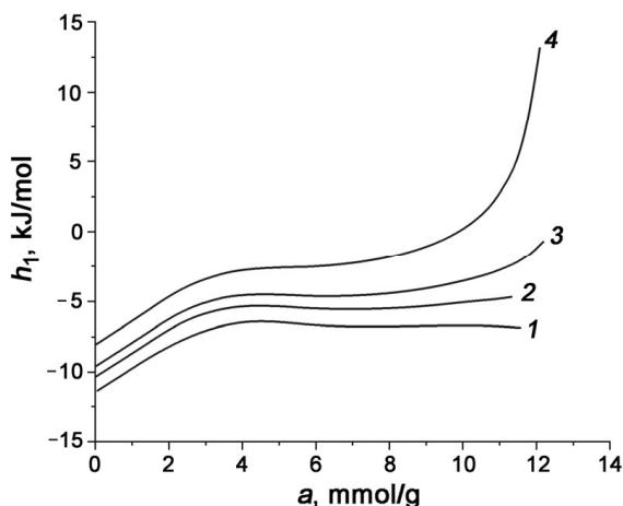
**Figure 9.** The differential molar enthalpy of the WNS-AC-2-CO<sub>2</sub> adsorption system versus the amount of adsorbed carbon dioxide at temperatures, K: 243.0 (1), 273.0 (2), 293.0 (3), and 333.0 (4).
