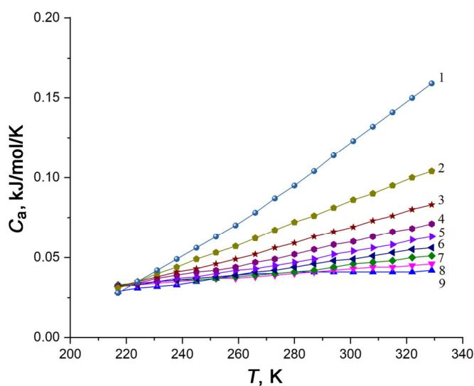
**Figure 11.** The differential molar heat capacity,  $C_a$ , of the WNS-AC-2-CO<sub>2</sub> adsorption system as a function of temperature for various CO<sub>2</sub> uptakes: 11 mmol/g (1), 10 mmol/g (2), 9 mmol/g (3), 8 mmol/g (4), 7 mmol/g (5), 6 mmol/g (6), 5 mmol/g (7), 4 mmol/g (8), and 3 mmol/g (9).
