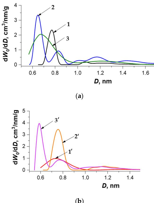
**Figure 3.** The PSD functions  $dW_0/dD = f(D)$  in two series of carbon porous materials prepared from WNS char (a) and HNS char (b) via KOH thermochemical activation with a char/KOH ratio of 1:1 (curves 1 and 1'), 1:2 (curves 2 and 2'), and 1:3 (curves 3 and 3').
