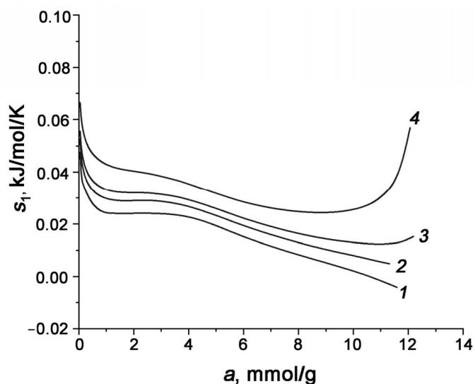
**Figure 10.** The differential molar isosteric entropy of the WNS-AC-2–CO<sub>2</sub> adsorption system versus the CO<sub>2</sub> uptake at temperatures, K: 243.0 (1), 273.0 (2), 293 (3), and 303.0 (4).
