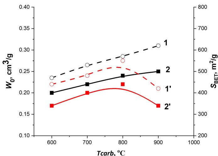
**Figure 1.** Dependence of the porous structure parameters:  $S_{\text{BET}}$  (dash curves 1, 1') and  $W_0$  (solid curves 2, 2') of the WNS char (black curves 1 and 2) and HNS char (red curves 1' and 2') samples on the carbonization temperature.
