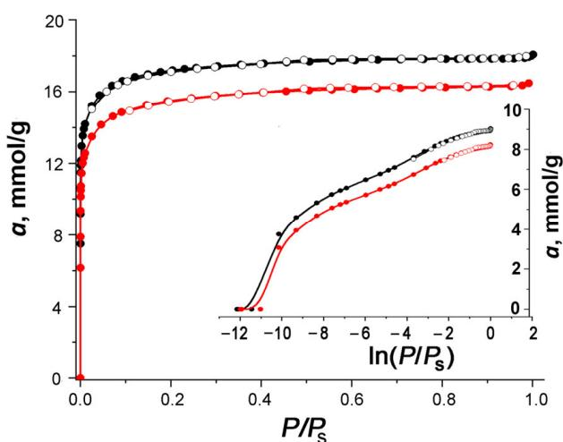
**Figure 2.** The standard isotherms of nitrogen vapor adsorption onto WNS-AC-2 (black symbols and lines) and HNS-AC-3 (red symbols and lines) measured at 77 K.
