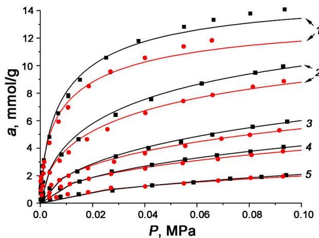
**Figure 7.** The initial part of the  $\text{CO}_2$  adsorption isotherms for the WNS-AC-2 (black) and HNS-AC-3 (red) samples up to pressures of 0.1 MPa at temperatures, K: 216.4 (1); 243.0 (2); 273.0 (3); 293.0 (4); 333.0 (5).
