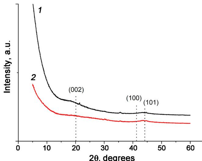
**Figure 5.** XRD patterns of the synthesized WNS-AC-2 (1) and HNS-AC-3 (2) adsorbents.
