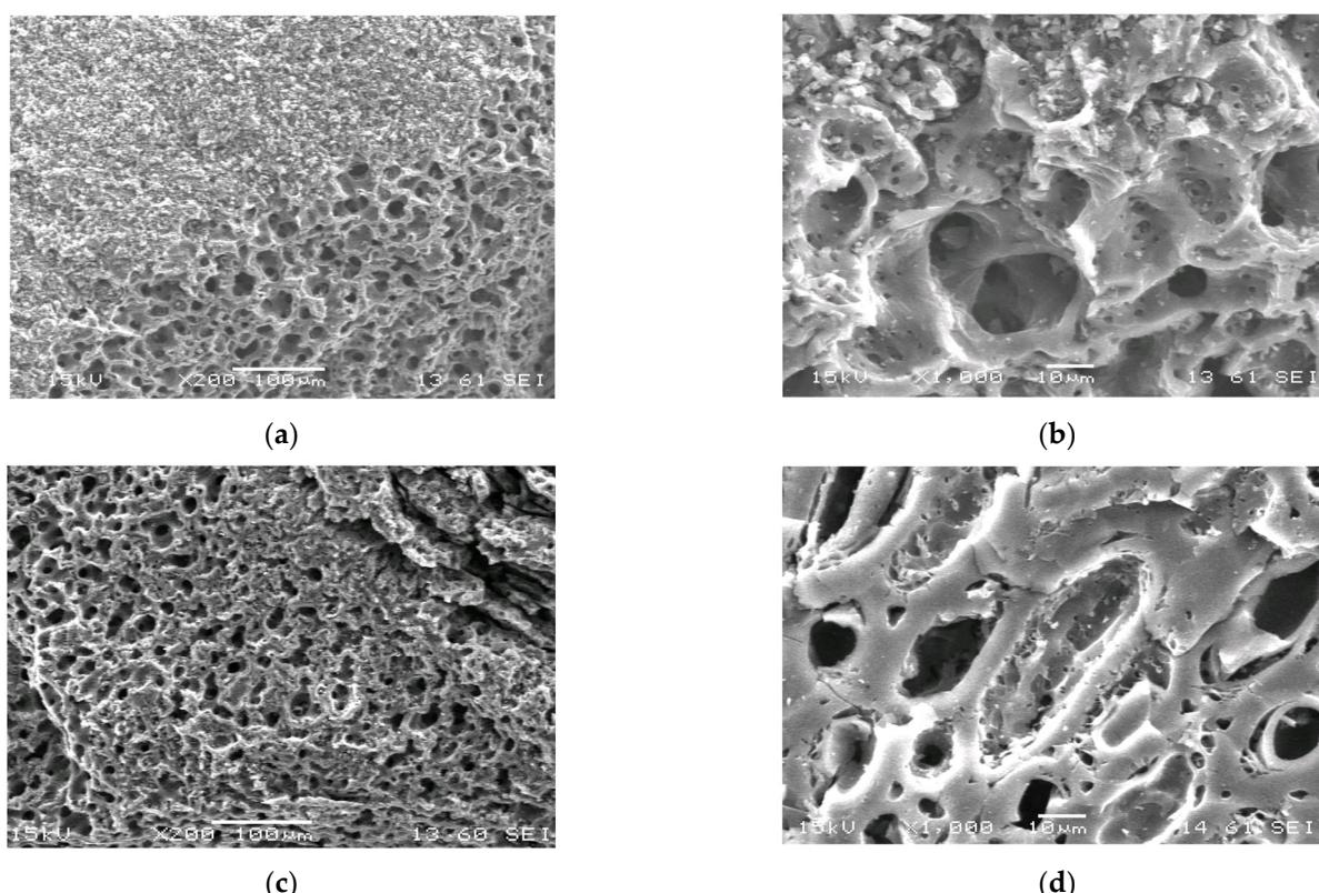
**Figure 4.** SEM images of the WNS-AC-2 (a,b) and HNS-AC-3 (c,d) carbon adsorbents.
