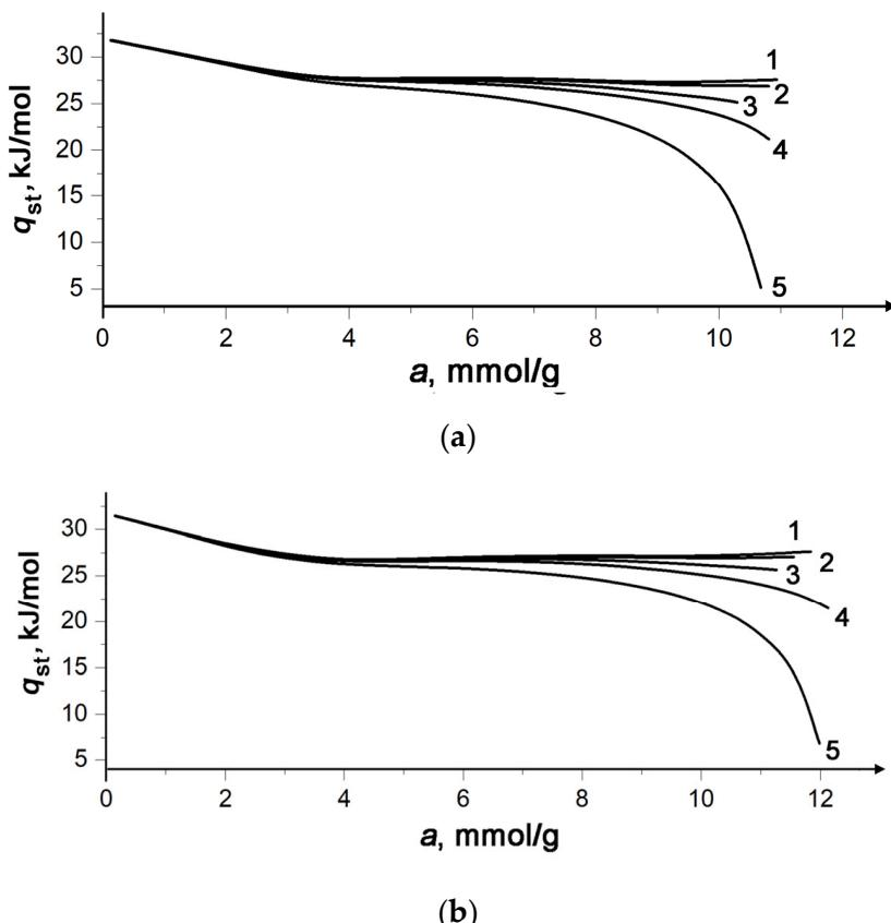
**Figure 8.** The differential molar isosteric heat of CO<sub>2</sub> adsorption onto WNS-AC-2 (a) and HNS-AC-3 (b) versus the adsorption value at temperatures, K: 216.4 (1), 243.0 (2), 273.0 (3), 293.0 (4), and 333.0 (5).
