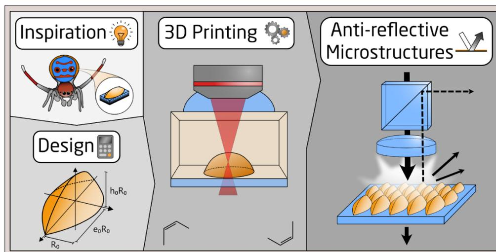
**Figure 2.** The fabrication and characterization of antireflective microarrays stimulated by the peacock spider's super-black structures encountered in nature. First: different microarray 3D models are produced from a surface equation. Second: the arrays are invented in a polyacrylate resin via super-resolution 3D printing through two-photon polymerization. Third: the bioinspired micro-lens arrays show excellent antireflective properties [61].
