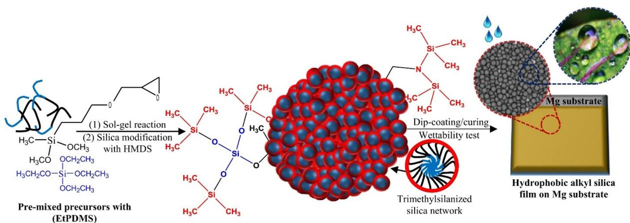
**Figure 1.** An illustrative preparation protocol of a bioinspired alkyl-silanized coating for Mg corrosion prevention reported in this study [47].
