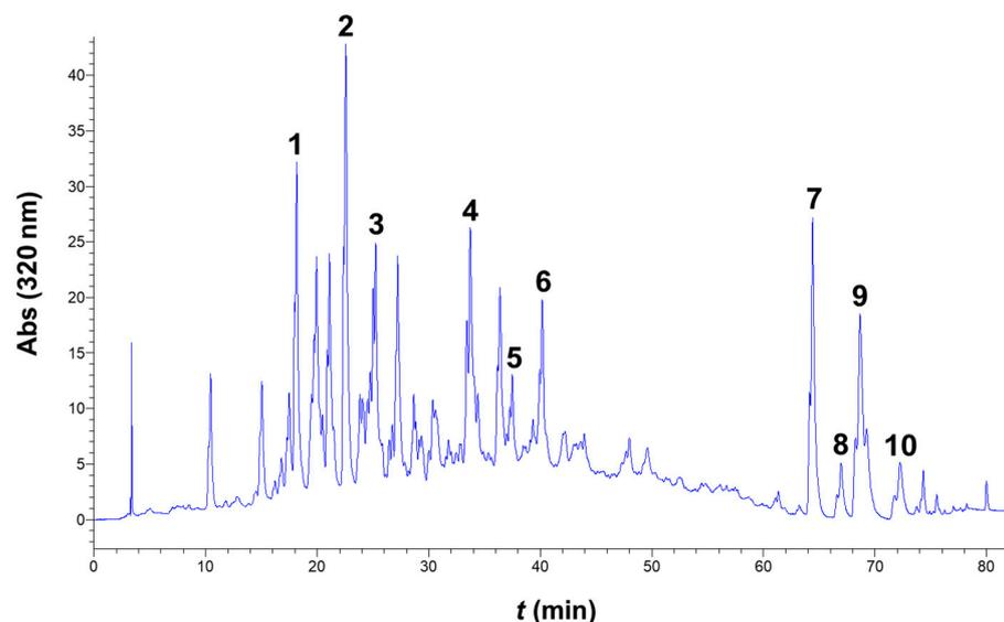
**Figure 7.** A representative chromatogram of a WOP extract produced using the optimal settings of the ultrasonication process (80% amplitude, 15 min). Peak assignment: 1, neochlorogenic acid; 2, chlorogenic acid; 3, caffeic acid; 4, ferulic acid; 5, narirutin; 6, hesperidin, 7, didymin; 8, sinensetin; 9, nobiletin; 10, dimethylnobiletin.
