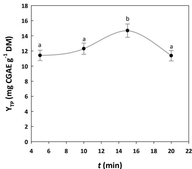
**Figure 2.** Effect of ultrasonication time on the yield in total polyphenols, during the aqueous extraction of waste orange peels at a constant amplitude of 75% and frequency of 50 Hz. The temperature variation during the extraction process varied was 14–19 °C. Designation with different small letters (a, b) shows statistically significant differences ( $p < 0.05$ ).
