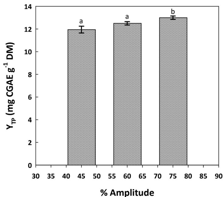
**Figure 1.** Effect of % amplitude of ultrasonication on the yield in total polyphenols, during the aqueous extraction of waste orange peels for 10 min, at a constant frequency of 50 Hz. The temperature variation during the extraction process was between 14–19 °C. Designation with different small letters (a, b) shows statistically significant differences ( $p < 0.05$ ).
