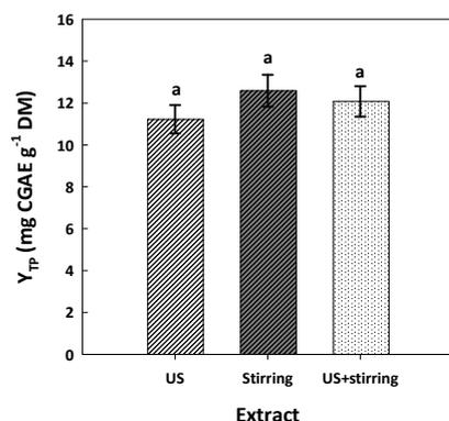
**Figure 5.** Effect of the various extraction modes tested on total polyphenol yield. Assignments: US, ultrasound-assisted extraction, performed under optimized settings (80% amplitude, 15 min); stirring, stirred-tank extraction performed under optimized setting (55 °C, 60 min); US and stirring, hybrid mode employing the ultrasound-assisted extraction as pretreatment, followed by the stirred-tank extraction. Assignment all columns with “a” denotes no statistical difference.
