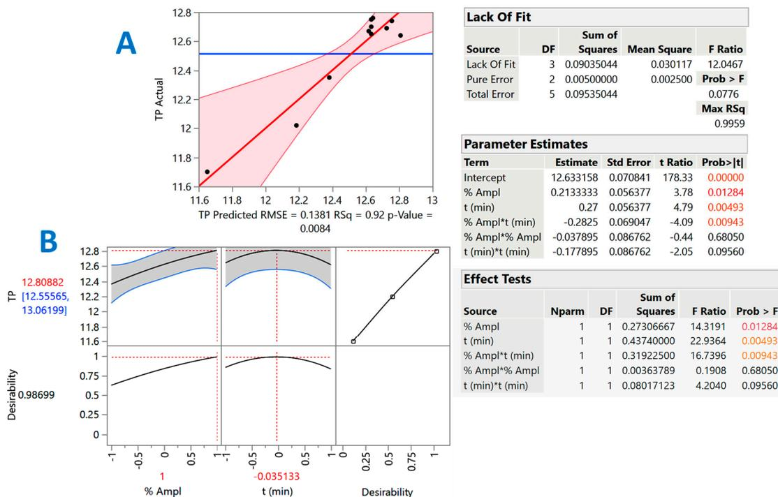
**Figure 3.** The actual vs. predicted values graph (A) and the graph depicting the desirability function (B). The inset tables present the analytical statistical data computed for the response surface optimization of the process. Values shown with different color are statistically significant (orange color,  $p < 0.01$ ; red color,  $p < 0.05$ ).
