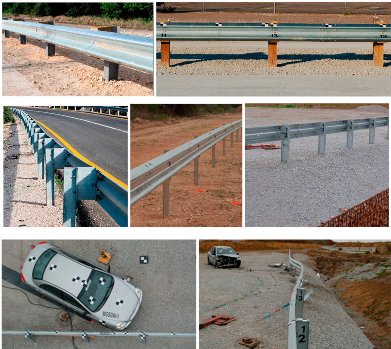
Figure 1. Various soil-embedded vehicle barrier systems for standard and special applications [4–6].
