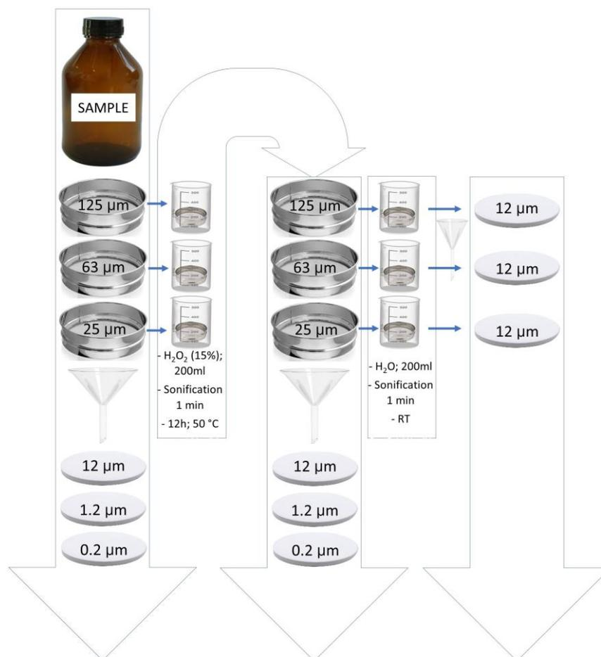
**Figure 4.** Scheme of different filter membranes and sieves used in proposed atmospheric MPs size fractionation from passive collector sample.
