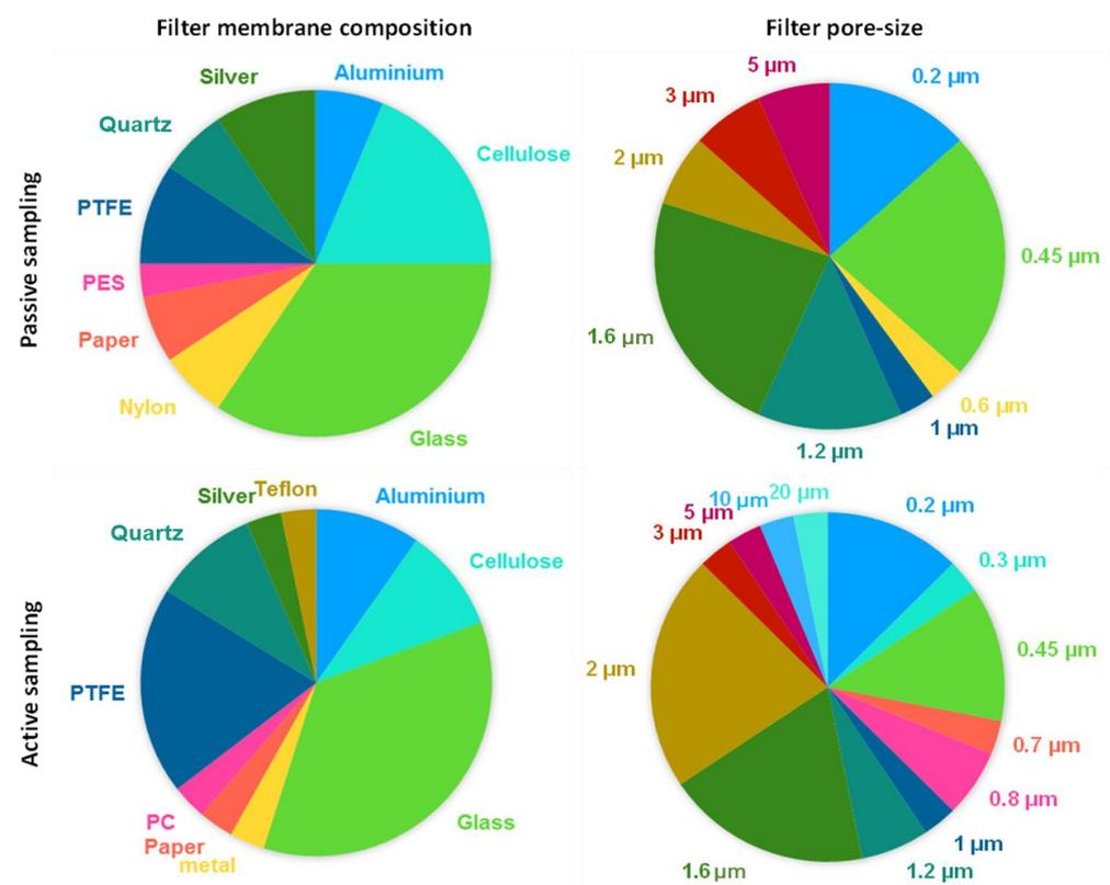
**Figure 3.** Different filter membrane compositions and pore sizes used in atmospheric microplastic sampling were reported in studies from 2020 to 2022.
