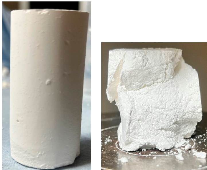
Figure 4. Functional plug sample obtained from 500–3000 ppm, or 1–6 mgpol/g \text{CaCO}_3 (left) and fractured plug sample obtained above 3000 ppm, or 6 mgpol/g \text{CaCO}_3 (right).
