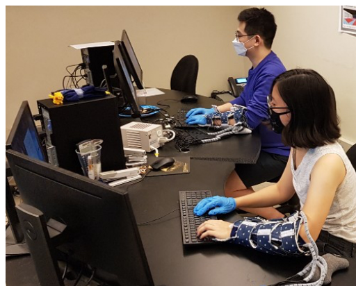
Figure 5. Photo of two-way messaging via TAPS. Each participant wore a TAPS system on the left forearm to receive text messages. They recorded received messages and sent new messages on computer keyboards.
