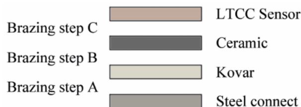
**Figure 9.** Diagram depicting the progressive integration process of an LTCC sensor into the steel connector.
