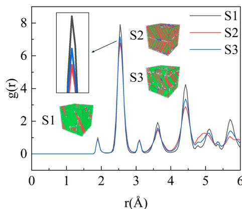
**Figure 2.** Radial distribution function [ $g(r)$ ] of the Cu/SiC composites cooled to 200 K.
