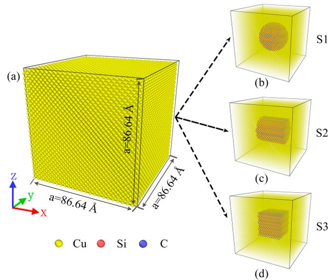
**Figure 1.** (a) Model diagrams of Cu/SiC composites, three models after copper atom transparency: (b) S1, (c) S2, and (d) S3.
