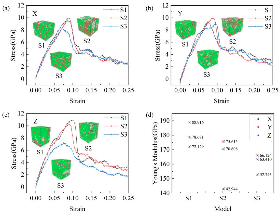
**Figure 9.** Stress–strain curves of three models stretched at 200 K for (a) X-axis, (b) Y-axis, and (c) Z-axis. (d) Young's modulus.
