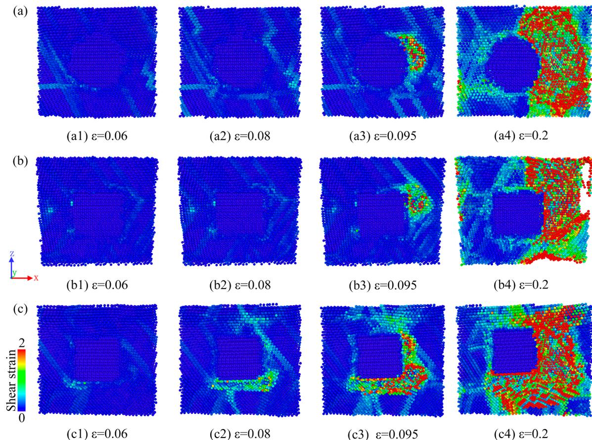
Figure 10. Deformation evolution of (a) S1, (b) S2, and (c) S3 models under X-axis stretching (slices).
