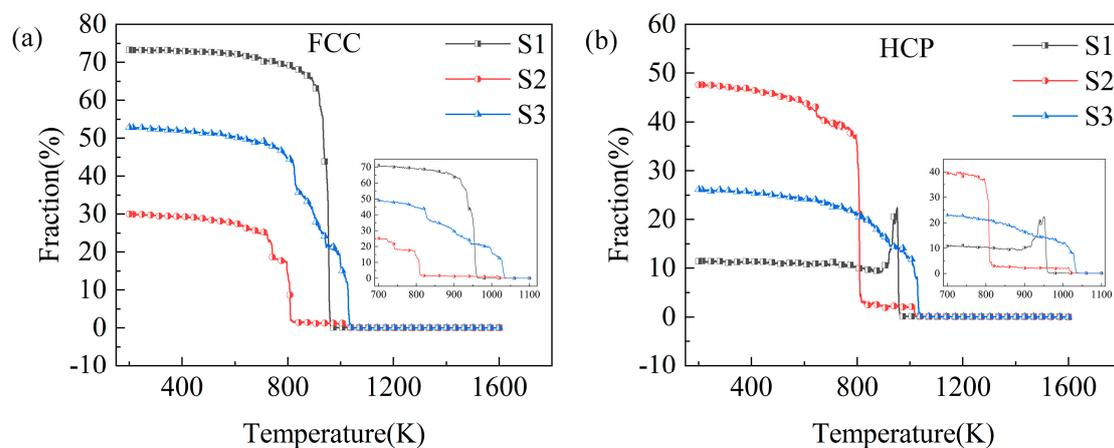
**Figure 4.** Volume fractions of FCC and HCP structures in different models at a cooling rate of  $10^{11}\text{ K}\cdot\text{s}^{-1}$ . (a) FCC structures, (b) HCP structures.
