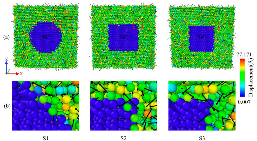
**Figure 3.** (a) The slice shows the change in the displacement of atoms in the three composite models. (b) is a magnified view of the interface in the red dashed box in (a). The black arrow pointing represents the direction of displacement, and the length represents the size of the displacement. Meanwhile, the closer the color is to red, the stronger the displacement is.
