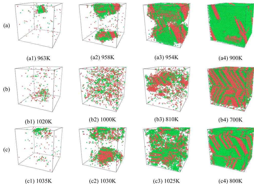
**Figure 5.** The structural evolution of FCC and HCP in different models. (a) S1, (b) S2, (c) S3. The green atoms are FCC structures, and the red atoms are HCP structures.
