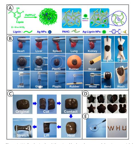
**Figure 9.** (**A**). Synthesis of multifunctional hydrogels as wound dressing materials based on lignin (light green), Ag nanoparticles (blue), and phenylboronic acid-modified hydroxypropyl cellulose (PAHC, gren). (**B**). Adhesion on organic and inorganic substrates. (**C**). Self-healing capability, (**D**). shape adaptivity, and (**E**). Demonstration of injectability of the created lignin-based hydrogels. Adapted with permission from ref. [270]. Copyright 2021, American Chemical Society.
