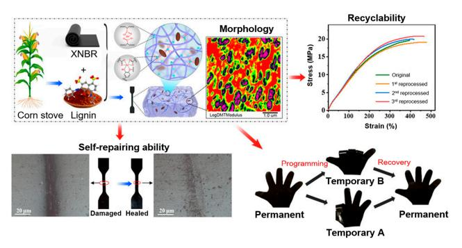
**Figure 11.** Multifunctionality in lignin-based thermoplastic elastomer composites. Reprinted with permission from ref. [308] Copyright 2022, American Chemical Society.
