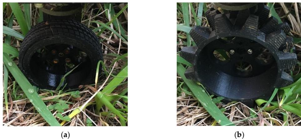
**Figure 12.** Wheels on grassy terrain. Wheel diameters are 60 mm, and the spike length is 10 mm. (a) Normal wheel. (b) Spiked wheel.
