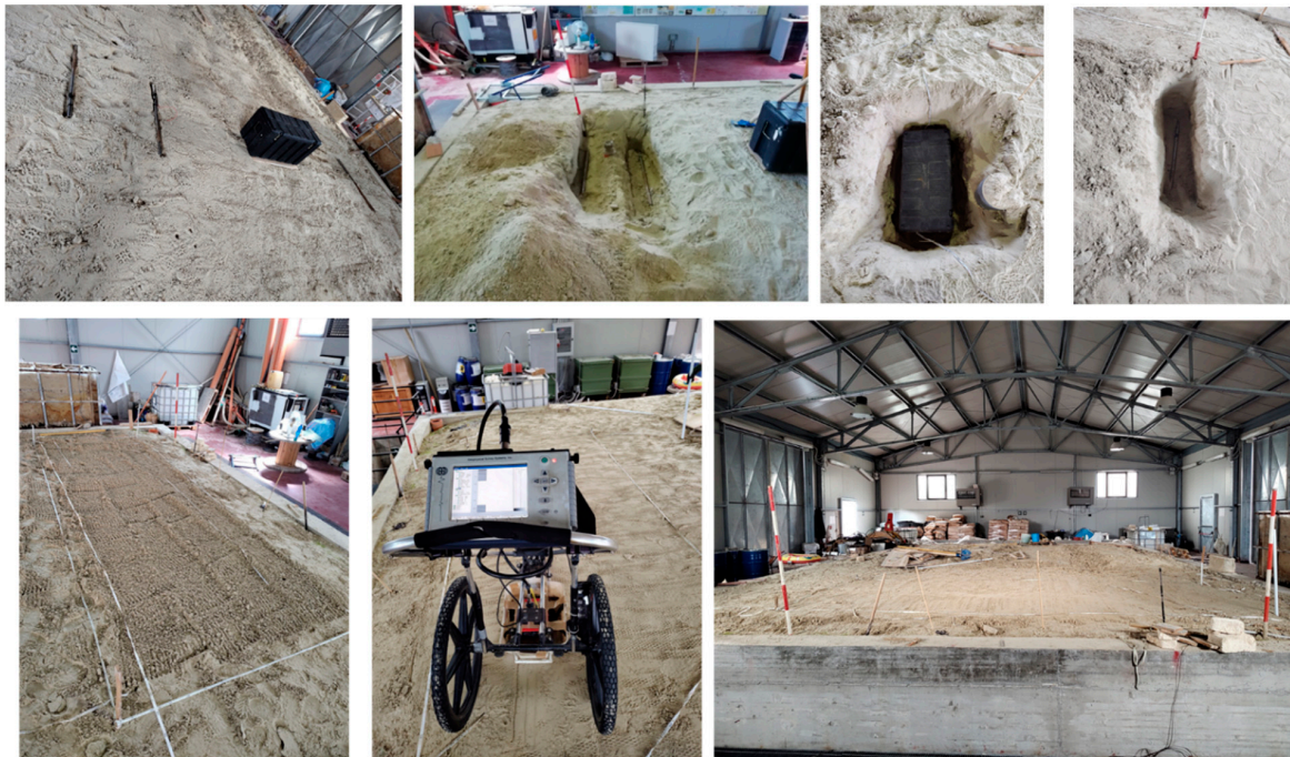
Figure 2. Set-up for the measurements with phases of the excavation for displacing the targets.
