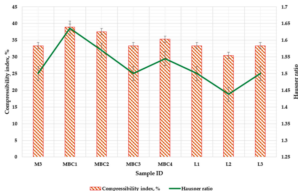
Figure 6. Assessment of compressibility (Carr index) and flowability (Hausner ratio) in spray-dried and freeze-dried powders formulated with varied wall materials. M3 (MD 10%, SK 10%); MBC1 (MD 13%, \beta -CD 5.8%, CMC 1.2%); MBC2 (MD 15%, \beta -CD 4.1%, CMC 0.9%); MBC3 (MD 17%, \beta -CD 2.5%, CMC 0.5%); MBC4 (MD 10%, SK 9%, \beta -CD 1%). L1 (MD 13%, \beta -CD 5.8%, CMC 1.2%); L2 (MD 15%, \beta -CD 4.1%, CMC 0.9%); L3 MBC3 (MD 17%, \beta -CD 2.5%, CMC 0.5%). M indicates the spray-dry method, and the L-lyophilization method is used.
