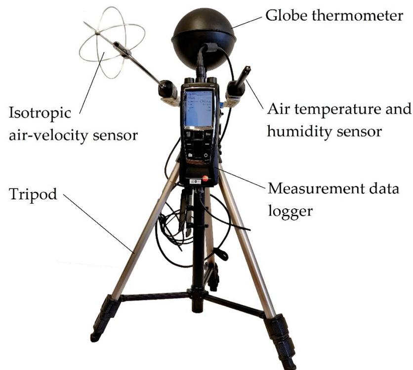
**Figure 2.** TESTO 480 multifunctional HVAC measuring instrument.
