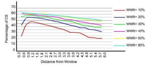
Figure 4. The relation between several WWRs and resulting CS values (adapted from [12]).
