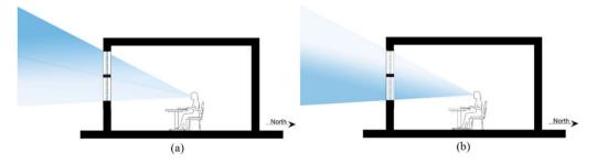
Figure 6. (a) Higher window admits more daylight under overcast sky; (b) lower window admits more daylight under clear sky.
