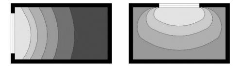
**Figure 3.** Luminous uniformity in rectangular space in relation to window placement within different facades.
