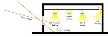
Figure 7. Different lighting schemes for indoor environments, provided by natural light and artificial light.
