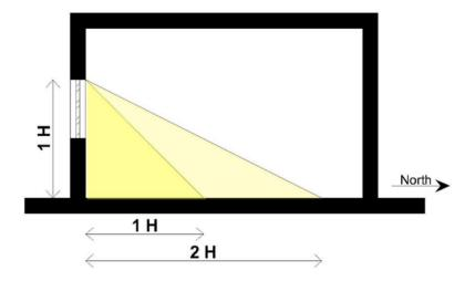
Figure 8. Window head height to light penetration depth rule of thumb.
