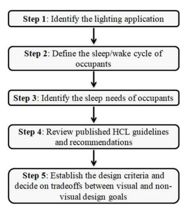
Figure 10. Design process proposed by Houser et al. (2021) for human-centric lighting.
