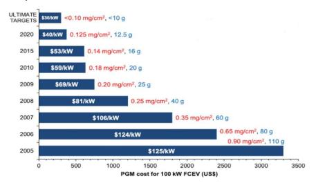
**Figure 8.** Cost and loading of platinum group metals (PGM) for 100 kW FCEV from 2005 to 2020, based on the current Pt raw price of USD  $\approx 30/g$ . The values inside the bars show the total fuel cell stack cost for a manufacturing volume of 500,000 units per year. The values outside the bars give the total catalyst loading per unit cell area (mg/cm<sup>2</sup>) and for a 100 kW FCEV (g). Adapted from [13].
