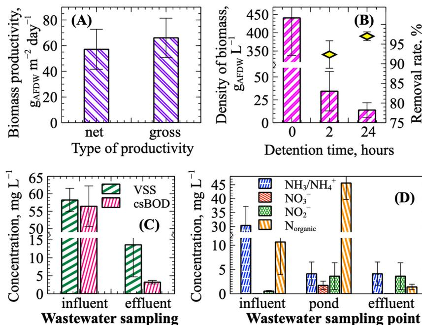
**Figure 1.** Average biomass productivity (A), biomass settling characteristics (yellow rhombus represents biomass removal rate) (B), and wastewater quality (C,D) throughout the cultivation study.
