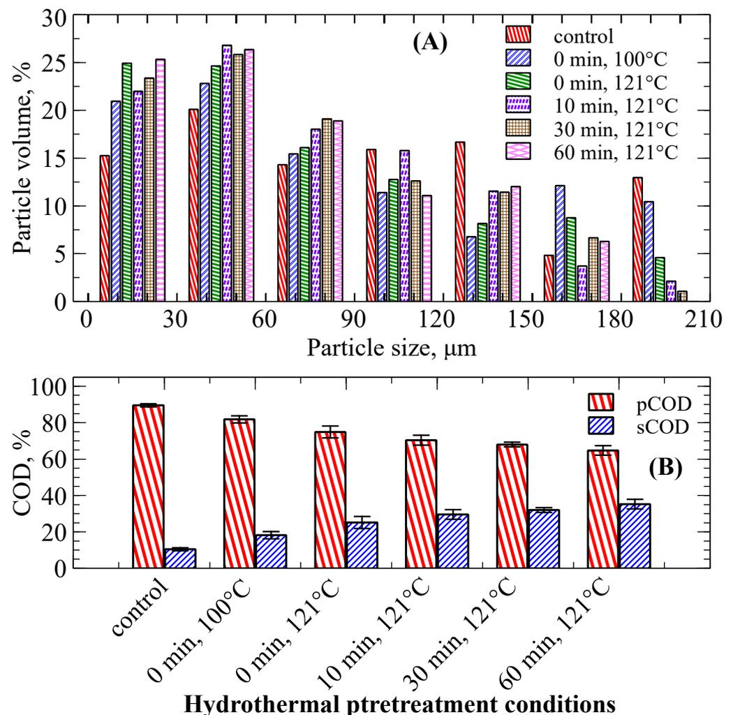
**Figure 3.** Distribution in algal biomass particle size (PSD) (A), and particulate vs. soluble chemical oxygen demand (pCOD and sCOD, respectively) (B). The particle size is reported as a volume equivalent sphere with diameter ranges of 0–30  $\mu m$ , 30–60  $\mu m$ , 60–90  $\mu m$ , 90–120  $\mu m$ , 120–150  $\mu m$ , 150–180  $\mu m$ , 180–210  $\mu m$ .
