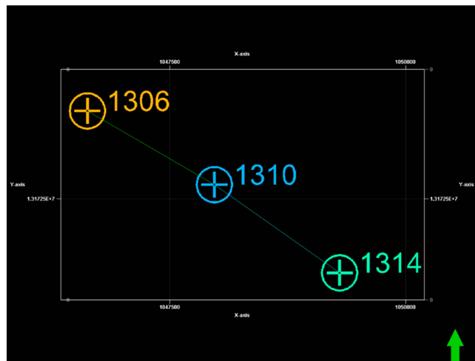
Figure 18. Geometry of the three wells used in the cross-well seismic tomography surveys. The arrow points north with the green side indicating the upward direction.
