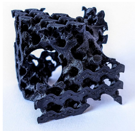
Figure 13. Recursive gyroid object printed by a FFF/FMD 3D printer from thermally conductive polymer composite filaments.
