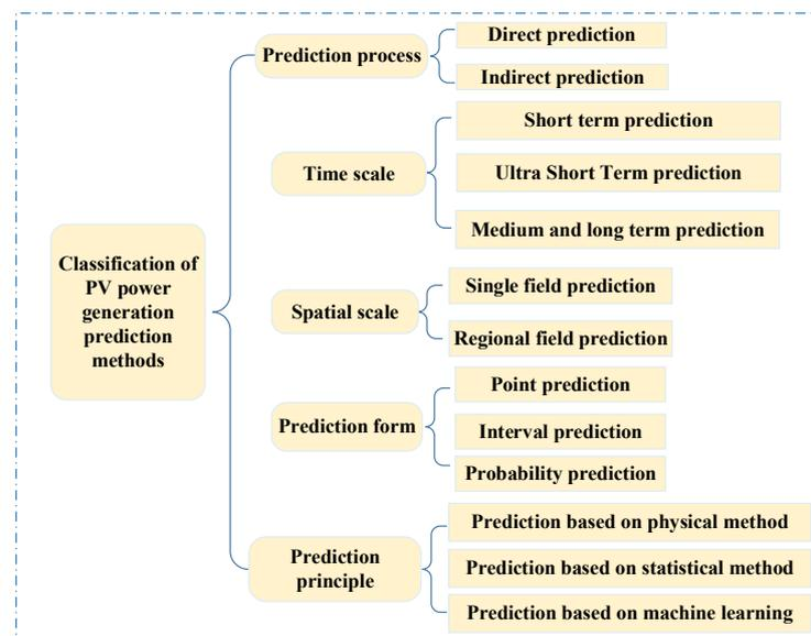
**Figure 1.** Classification of PV power prediction methods.
