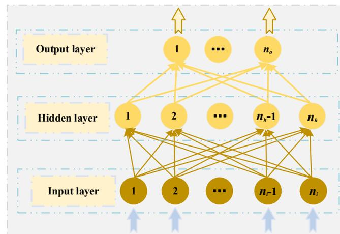
Figure 2. The network structure of ELM.
