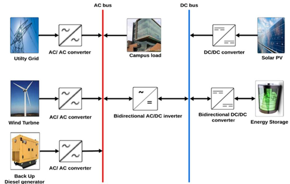
Figure 19. Microgrid connected with solar PV, WT, and ESS.
