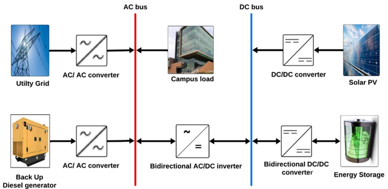
Figure 18. Grid connected with solar PV and energy storage.
