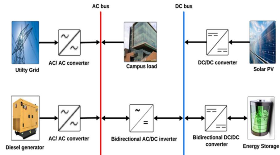
Figure 20. Grid connected with PV, diesel generator, and energy storage.
