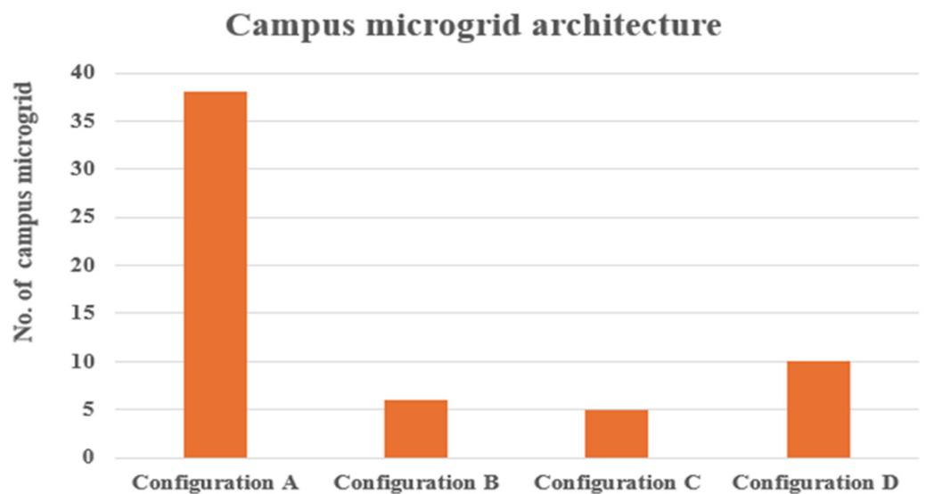
Figure 22. Comparison of the configurations, where configuration A is (Hybrid PV-grid-connected), configuration B is (Hybrid PV-WT-grid-connected), configuration C is (Hybrid PV-diesel generator-grid-connected), and configuration D is (Hybrid PV-CHP-grid-connected).
