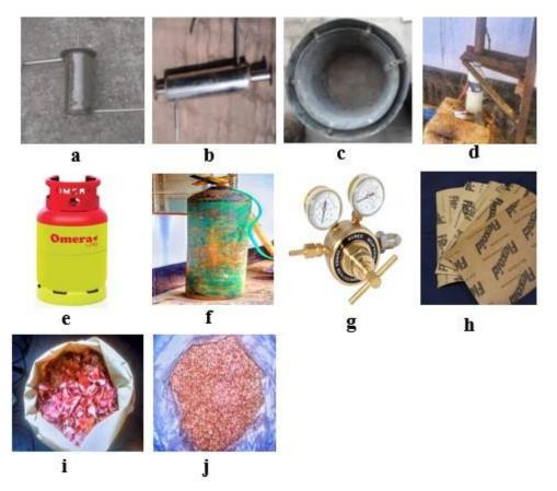
**Figure 1.** Different parts of the fixed-bed pyrolysis setup; (**a**) Reactor; (**b**) Condenser; (**c**) Biomass heater; (**d**) Liquid collector; (**e**) LPG cylinder; (**f**) N<sub>2</sub> gas cylinder; (**g**) MUREX 57 series gas flow meter; (**h**) Liquid gasket; (**i**) Onion shell; (**j**) Feed materials with average particles size of 200–300 μm.
