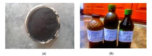
Figure 3. (a) Produced char. (b) Produced oil from onion shell pyrolysis.
