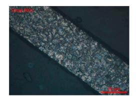
**Figure 19.** #Brut 1. Grain index (ASTM E112-13) G = 11.
