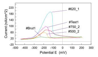
Figure 20. Potentio kinetic reactivation curves recorded for #Brut 1, #Test 1, #500\_1, #620\_2, and #750\_2.
