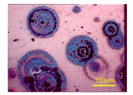
Figure 11. Corrosion pits revealed as blue discs (cross section sample #2).
