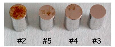
Figure 5. Uniform corrosion salt fog test, according to ASTM B 117-97. Samples #2-1.4427 So, #3-1.4435/316L, #4-316LUgim and #5-316L Val.
