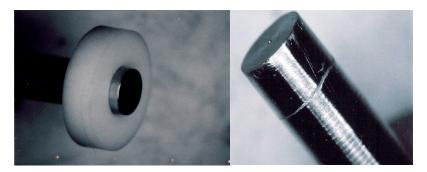
Figure 1. Specific assembly for the crevice corrosion test. Crevice corrosion aspect of the test sample.
