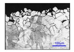
Figure 17. Metallographic section of the tube (#3, 1.4435/316L steel) after Strauss's test.
