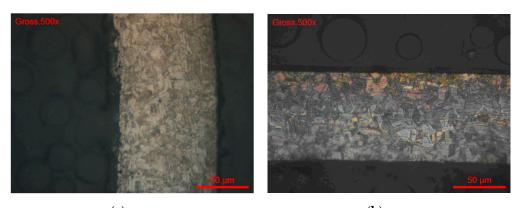
(a) (b) Figure 18. (a)#Test 1 and (b) #Test 2. Grain index (ASTM E112-13) G = 11.
