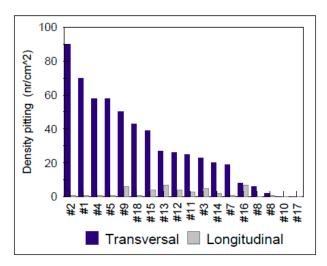
**Figure 6.** Pitting test results of the transverse and longitudinal surfaces for various grades of steel alloys (0.5 M FeCl<sub>3</sub> test medium at 50° for 2 h).
