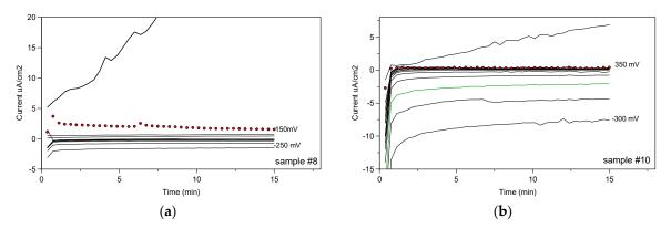
Figure 12. The crevice test potentiostatic curves for the longitudinal surface of sample #8 (a) and #10 (b).
