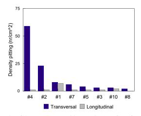
**Figure 7.** Pitting test results of the transverse and longitudinal surfaces for various grades of steels (0.1 M FeCl<sub>3</sub> test medium at 37 °C for 15 days).
