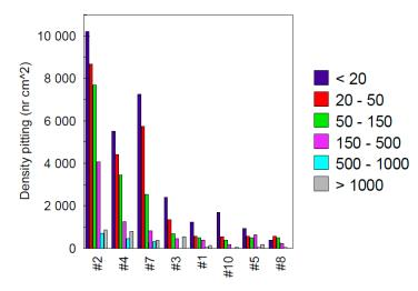
Figure 10. Number of pits counted by class, according to the size of the pit surface area.
