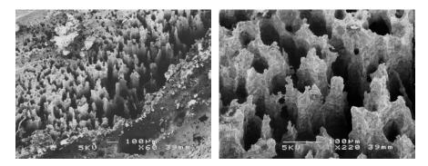
**Figure 15.** Scanning electron microscopy (SEM) of the transverse surface, corroded under a defective PTFE collar. The columnar morphology suggests preferential longitudinal dissolution due to the texture of the material.
