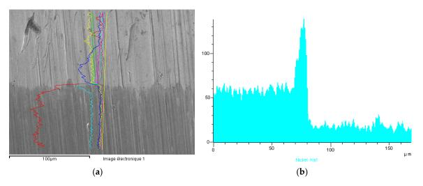
**Figure 25.** Sample #4. (a) EDX profiles of the gold-316 LM steel solder for iron, nickel, silver, gold, copper and zinc; (b) EDX Ni profile.
