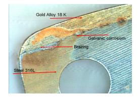
Figure 22. Galvanic corrosion in a gold-steel assembly.
