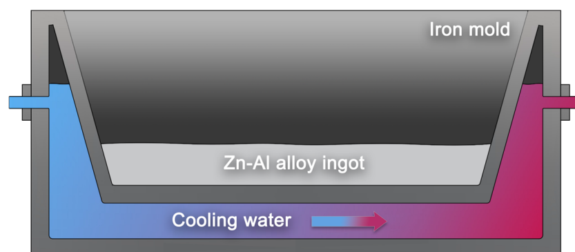
Figure 2. Cross-sectional diagram of water-cooled iron mold.
