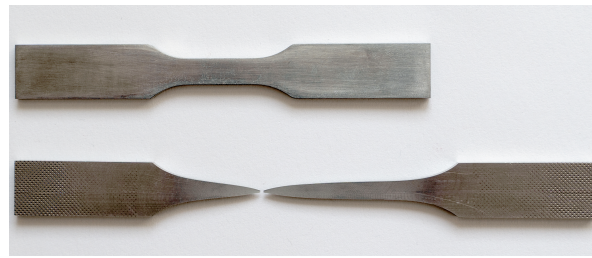
Figure 7. Specimens both before and after the monotonic tensile test.
