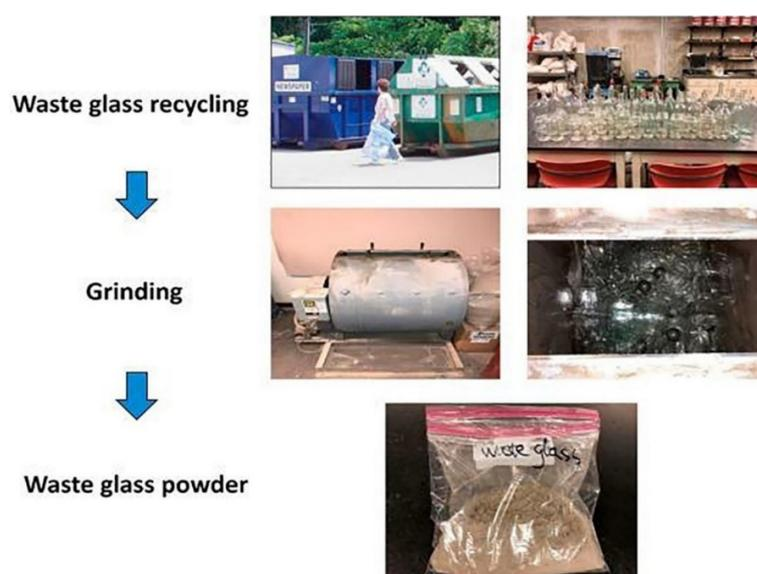
Figure 1. Simplified glass powder production process [25].
